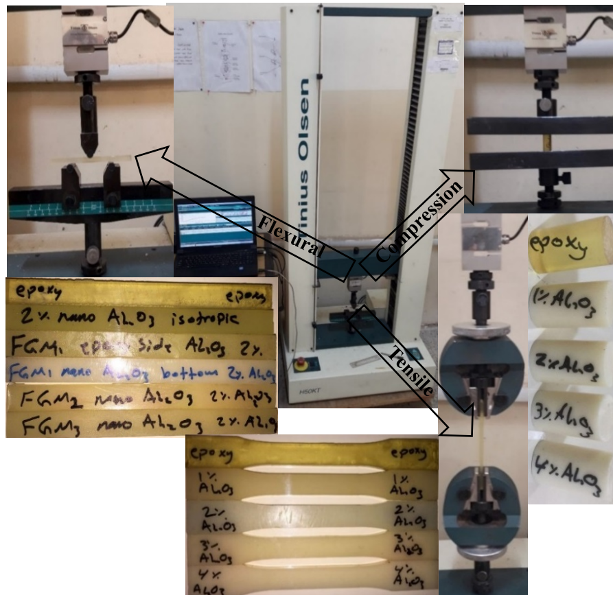
Figure 4: Universal testing machine and samples used
