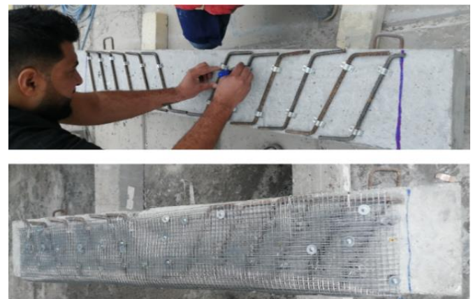
Fig. 7 The configuration of the externally bonded steel rebars used in the strengthening of the beam (S.-J. + Ferrocement + R).
