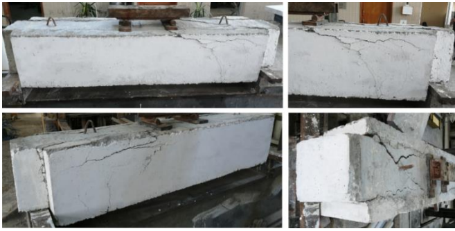
Fig. 12 The (S.-J. + Stirrup) beam after the Testing.
