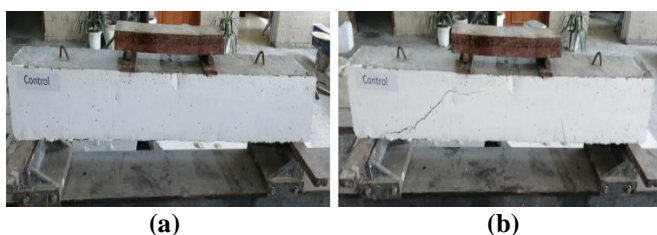
Fig. 10 The control beam (a) before the test and (b) after the failure.
