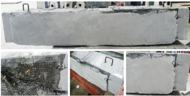
Fig. 13 The (S.-J. + Ferrocement) beam after the failure.
