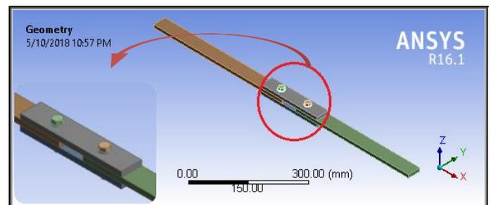
(c) Double lap bolted joint
