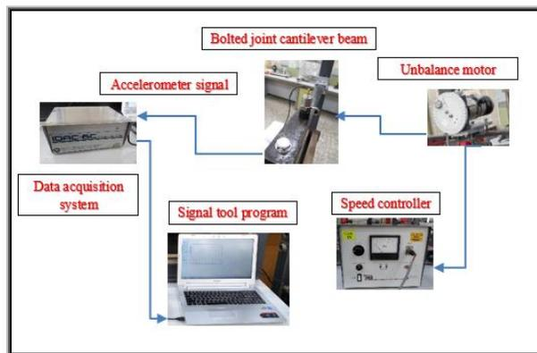
Fig.8 Experimental setup for forced vibration
