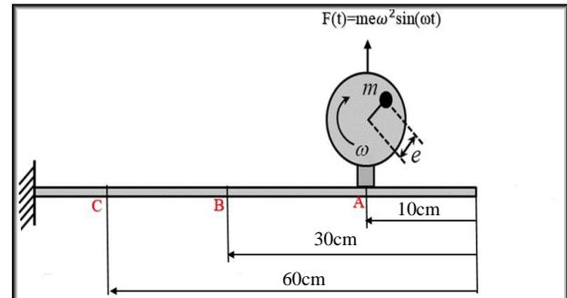
Fig.9 motor's positions on the cantilever beam
