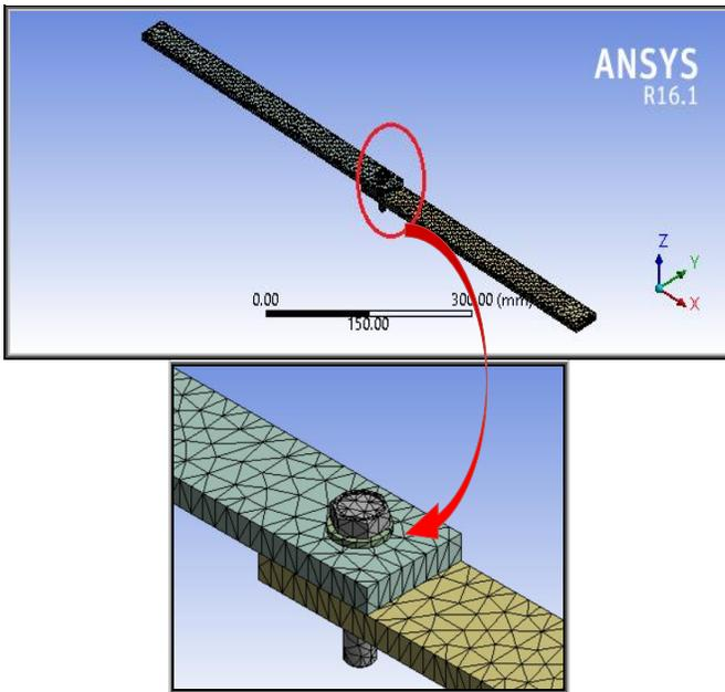
Fig.15 Meshing of bolted joint assembly
