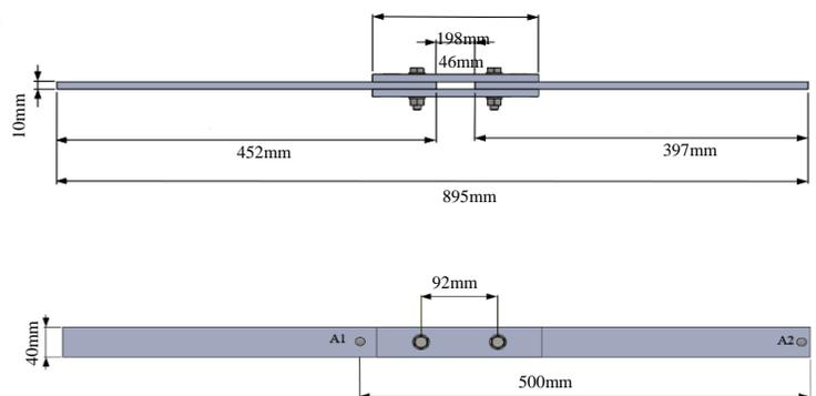
Fig. 3 Double lap joint with sensor locations (front and top view)
