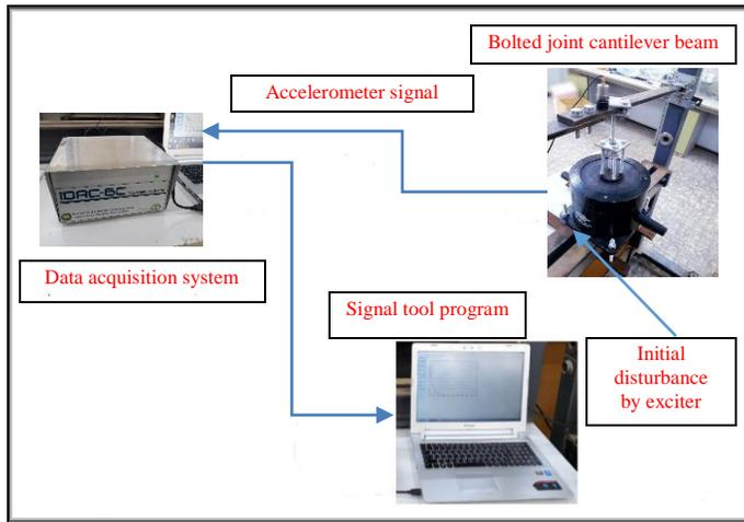
Fig. 5 experimental setup for free vibration
