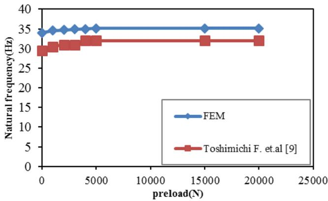
Fig.18 effect of preload on natural frequency
