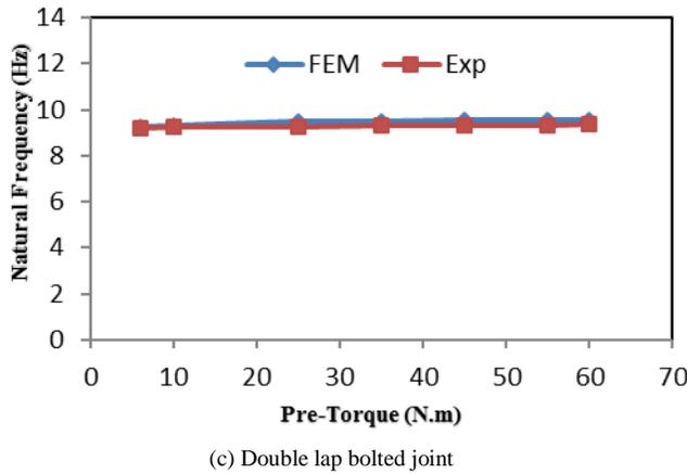
Fig.22 Effect of preload on natural frequency for different beam configuration
