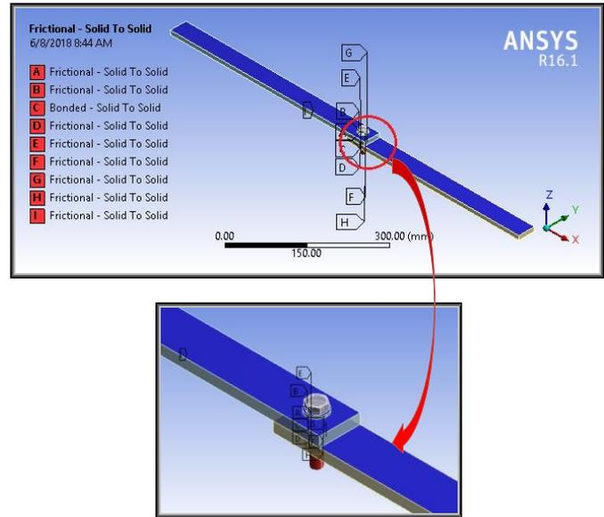
Fig.16 assembly with preferred contact
