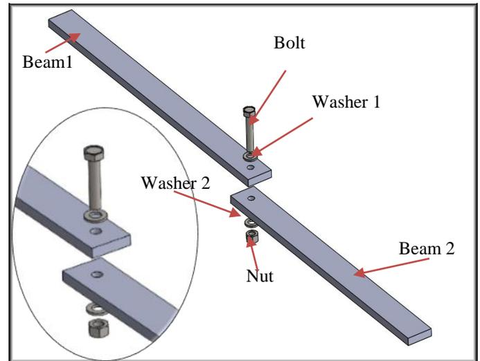
Fig.13 Bolted joint structure
