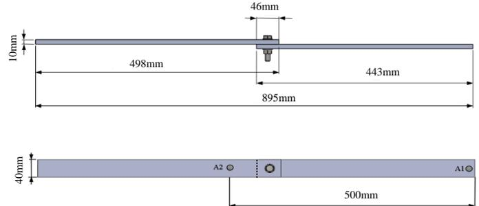
Fig.1 single lap joint with sensor location (front and top view)
