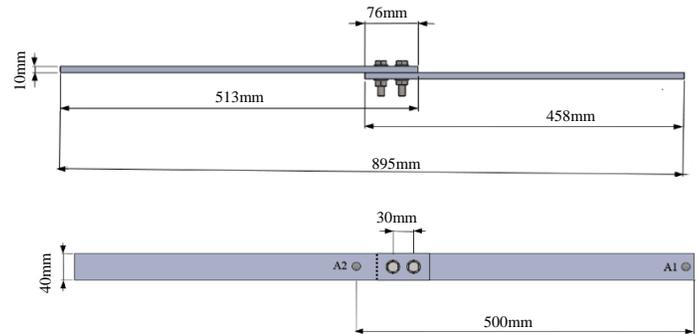
Fig.2 Double bolted lap joint with sensor location (front and top view)
