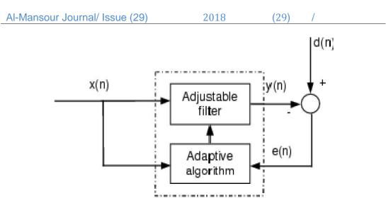
Figure (1) Block Diagram of General Adaptive Filter
