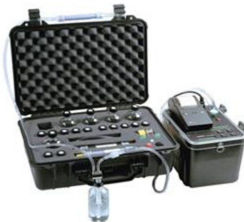
Figure (2) on the right is a picture of the RAD7 device used to measure radon in water models, and on the left is the RADH2O diagram.
