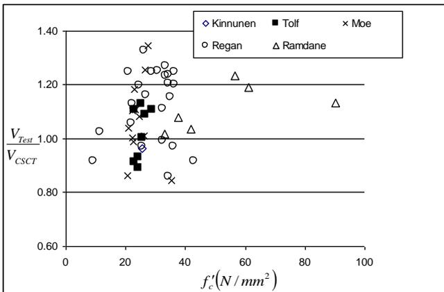
(c)  $\frac{V_{Test}}{V_{CSCT}}$  for tests with aggregate type of gravel
