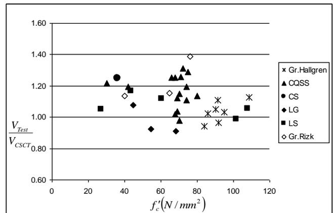
(c)  $\frac{V_{Test}}{V_{CSCT}}$  for tests with various types of aggregate
