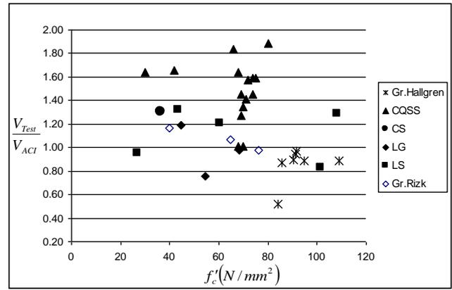
(a)  $\frac{V_{Test}}{V_{ACI}}$  for tests with various types of aggregate
