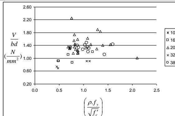
Fig. 7 Strength of slabs with gravel aggregate
