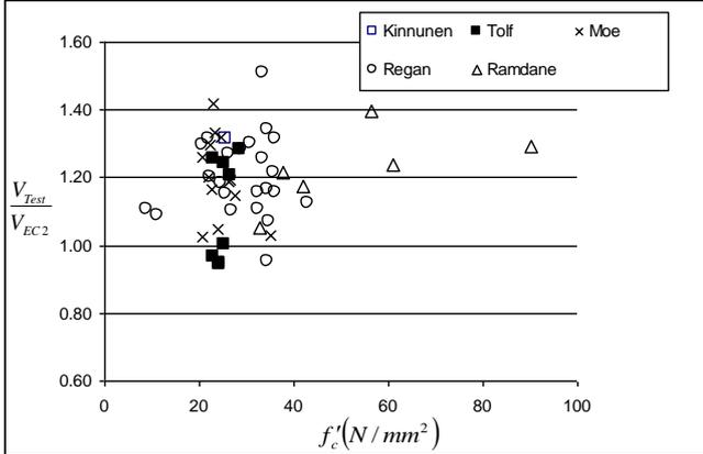
(b)  $\frac{V_{Test}}{V_{EC2}}$  for tests with aggregate type of gravel
