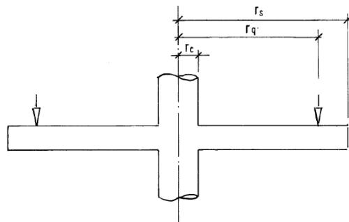
Fig. 2. Definition of  $r_c$ ,  $r_q$  and  $r_s$  by CSCT
