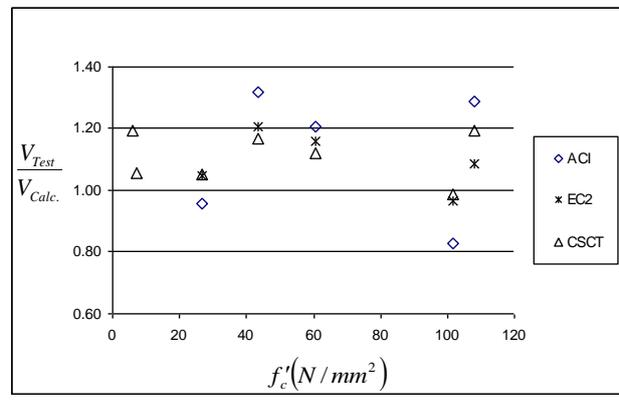
Fig. 6 Comparison of  $\frac{V_{Test}}{V_{Calc}}$  for limestone aggregate
