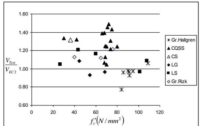
(b)  $\frac{V_{Test}}{V_{EC2}}$  for tests with various types of aggregate
