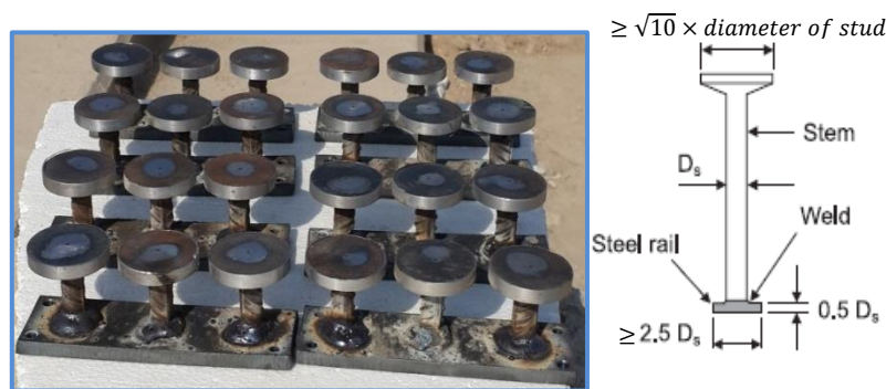
Fig. 3:- Configuration of shear studs.
