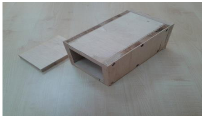
Figure (1): The form of the prepared mould
