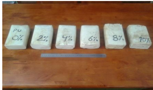
Figure (2): Polyurethane foam with glass wool fibers at a range of (0-10) % wt.
