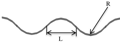
Fig.19. Geometry of sinusoidal corrugation [7]
