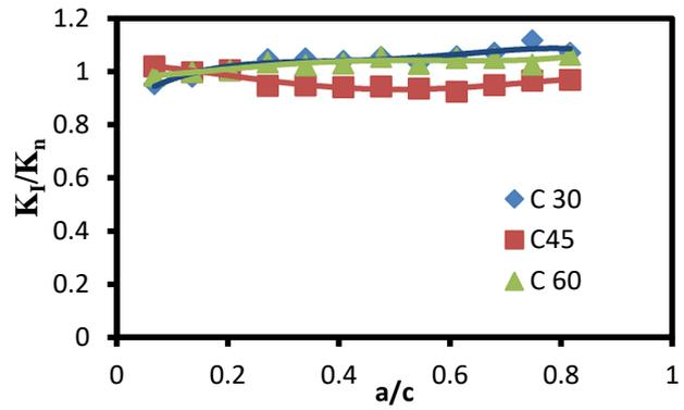
Fig. 16 .Effect of crack length on shape factor
