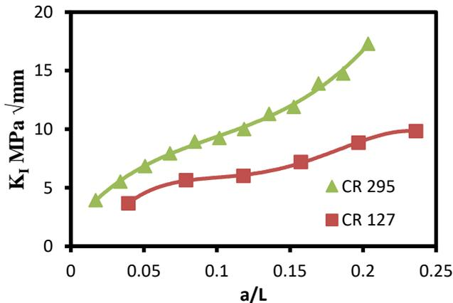
Fig. 20. Effect of crack length on the stress intensity factor
