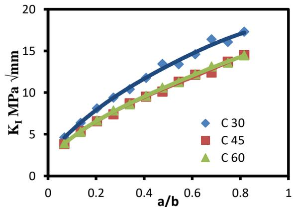
Fig.12. Effect of crack length on the stress intensity factor
