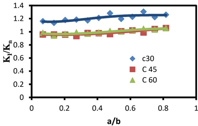
Fig13. Effect of crack length on shape factor
