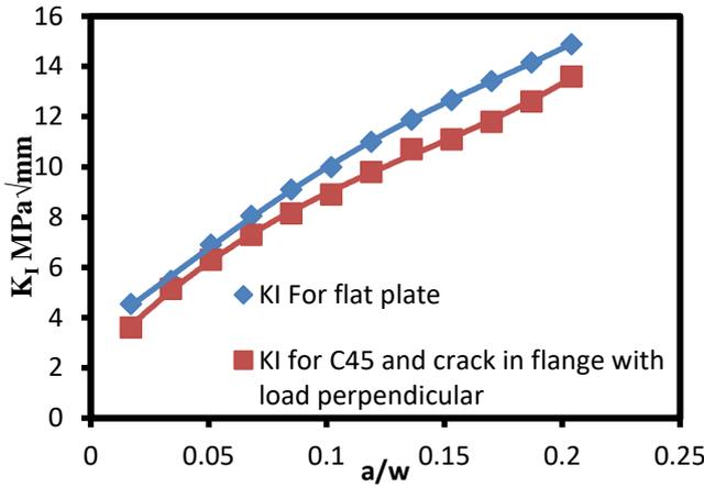
Fig.4. Effect of crack length on the stress intensity factor
