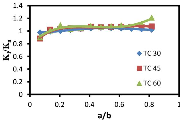
Fig28 . Effect of crack length on the shape factor.
