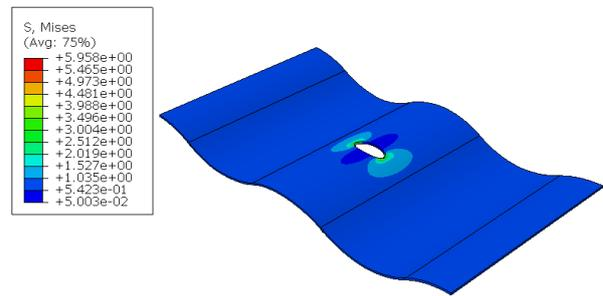
Fig. 22a Stress distribution fringes for curvature radius R 295 mm
