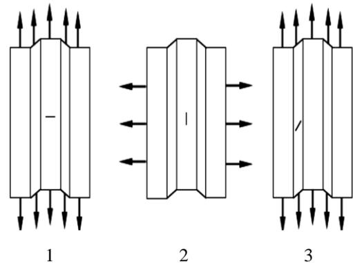
Fig.7. Crack location and load direction for each case
