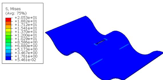
Fig. 25b Stress distribution fringes of R 127mm
