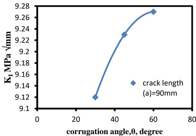
Fig29. Effect of corrugation angle on the stress intensity factor
