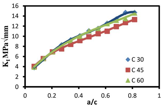
Fig. 15. Effect of crack length on the stress intensity factor
