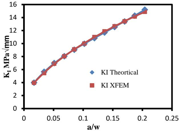
Fig. (3). Effect of crack length on the stress intensity
