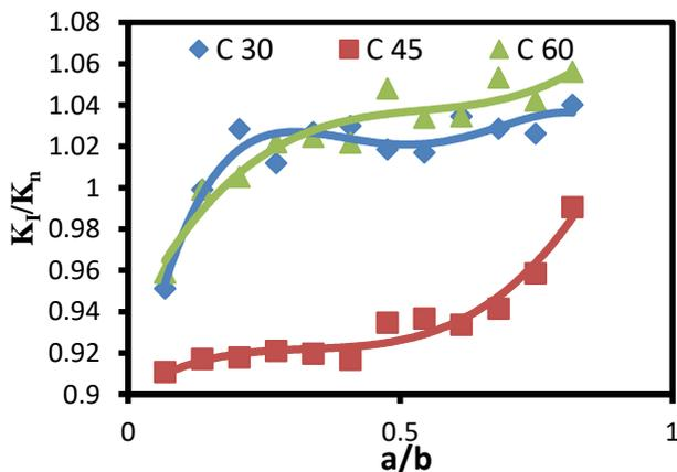
Fig. 10. Effect of crack length on shape factor
