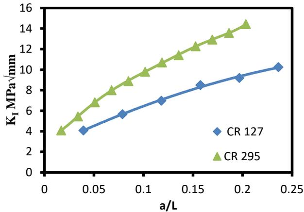
Fig. 23 Effect of crack length on the stress intensity factor
