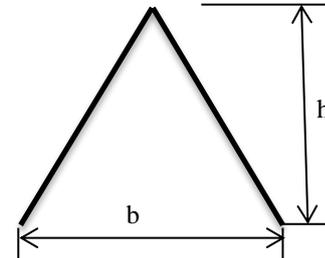
Fig. 26. Geometry of triangle corrugated plate
