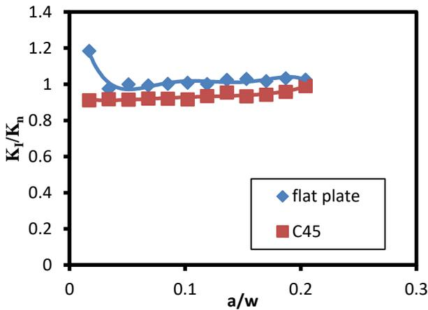
Fig.5. Effect of crack length on the shape factor
