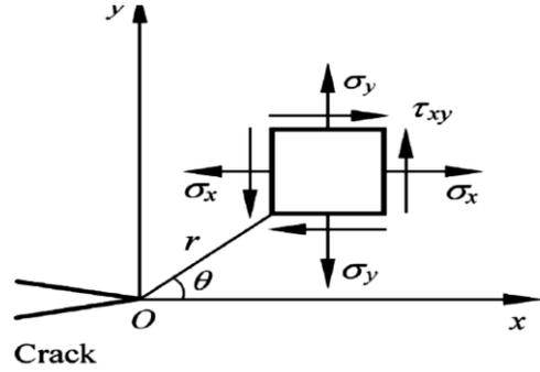
Figure1. Stress element at the crack tip
