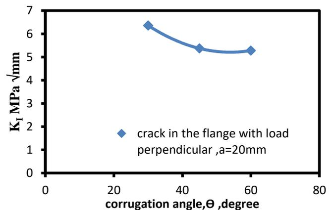
Fig. 18. Effect of corrugation angle on the stress intensity factor
