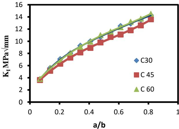
Fig. 9. Effect of crack length on the stress intensity factor  $K_I$
