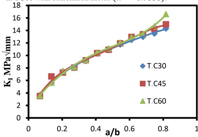
Fig. 27 . Effect of crack length on the stress intensity factor
