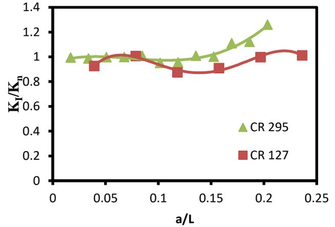
Fig. 21. Effect of crack length on shape factor
