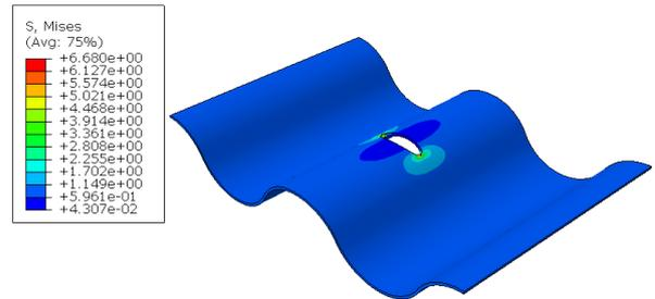
Fig. 22b Stress distribution fringes for curvature radius R 127 mm
