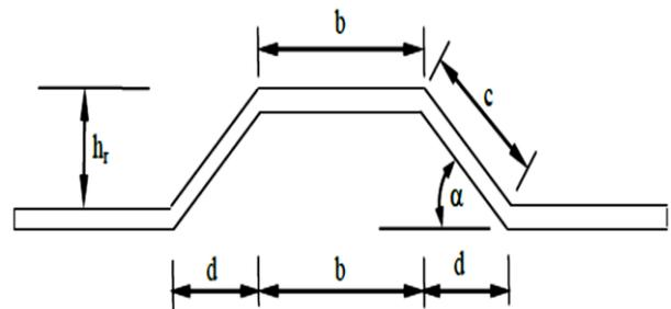
Fig.8. Geometry of corrugated plate [7]
