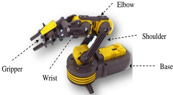
Fig.11 Body of the robot manipulator
