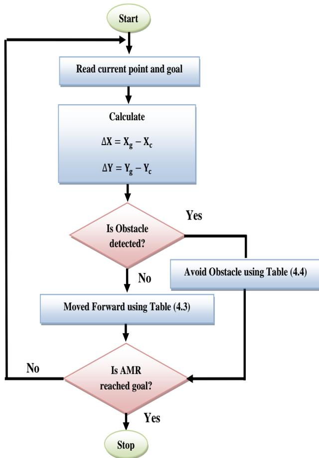
Fig. 6 Flowchart the motion control with GRFC and OAFC
