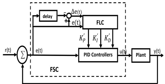
Fig. 2 Basic structure of FSC.
