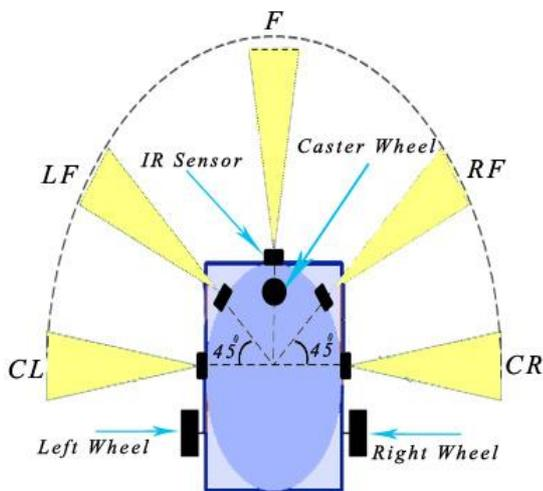
Fig. 1 The Autonomous Mobile Robot Platform
