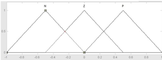
Fig.4(a): Membership Function of Error input for FSC.
