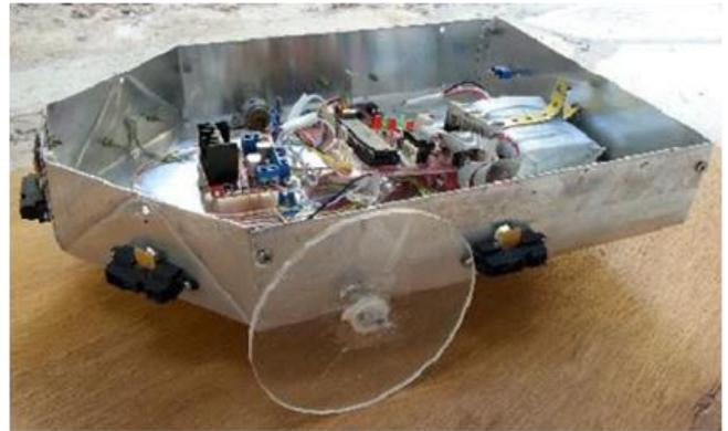
Figure (9): The designed autonomous mobile robot.
