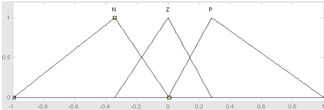
Fig.4(b): Membership Function change of Error input for FSC.
