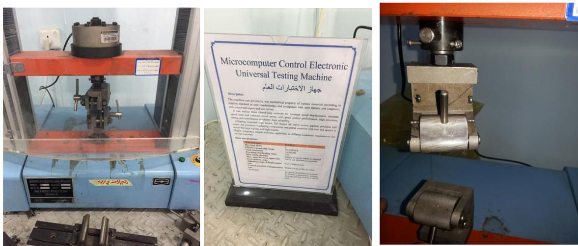
**Fig.(7). Testing machine of fiber wire mesh**
