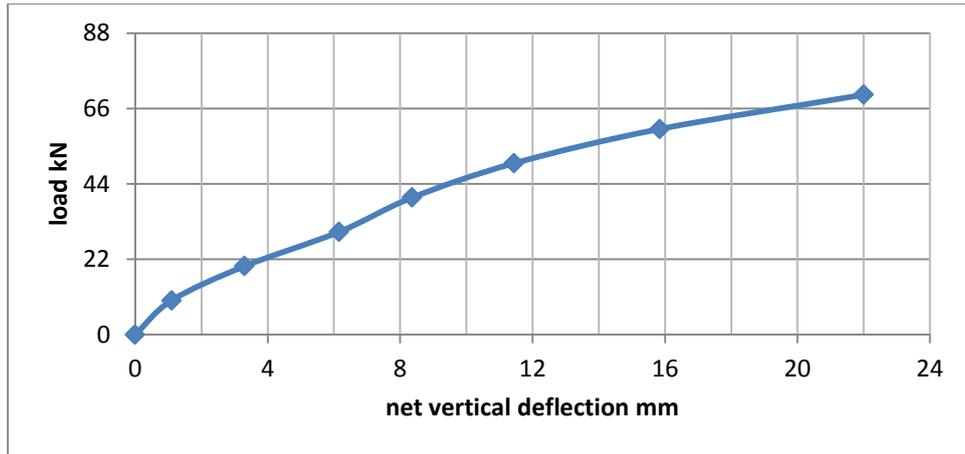
**Fig.(9).** Load vs net vertical deflection of RC beam S
