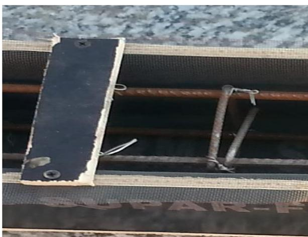
**Fig.(4). Fiber wire mesh inside wood mold**
