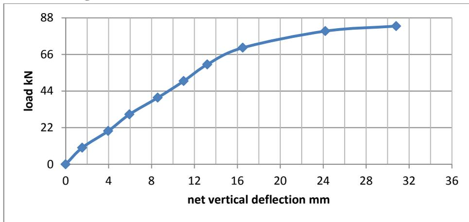
**Fig.(10).** Load vs net vertical deflection of RC beam SU
