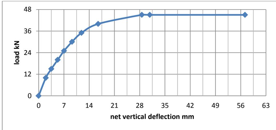
**Fig.(15).** Load vs net vertical deflection of RC beam FA
