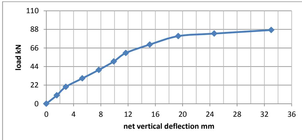
**Fig.(11).** Load vs net vertical deflection of RC beam SA
