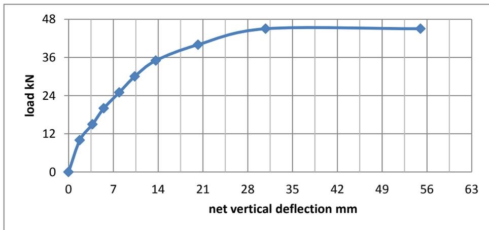
Fig.(14). Load vs net vertical deflection of RC beam FU
