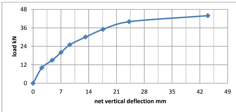
Fig.(13). Load vs net vertical deflection of RC beam F
