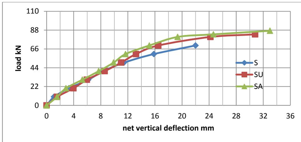
Fig.(12). Load vs net vertical deflection of RC beams S,SU and SA
