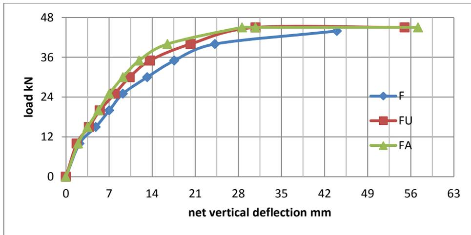
**Fig.(16).** Load vs net vertical deflection of RC beams F, FU and FA
