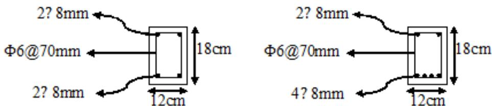
**Fig.(2). Cross-section of test specimen**
