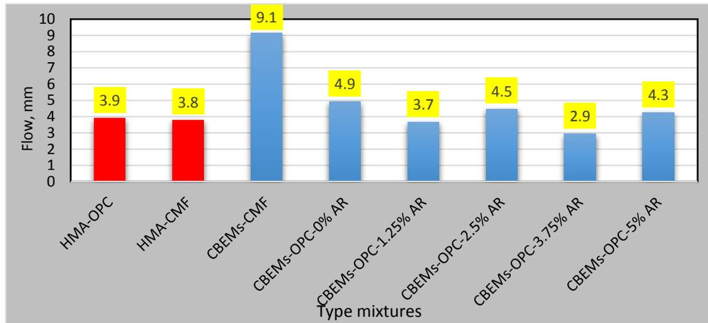
**Figure 3 Marshall Flow for asphalt mixtures**
