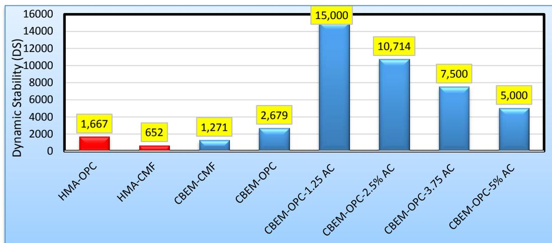
Figure 6 Dynamic Stability for CBEMS Comprising OPC-AR polymer
