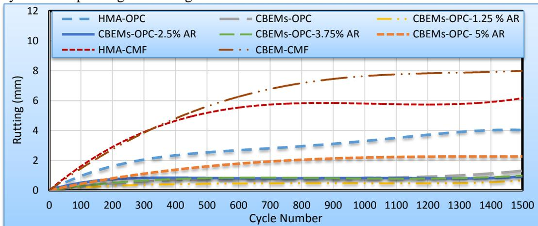
**Figure 5 Rutting Depth verse Cycle Number for CBEMs comprising OPC-AR polymer**
