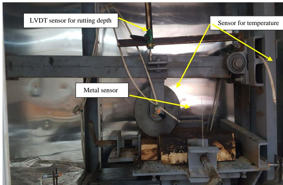
**Plate 3 Apparatuses for Wheel Track Device**
