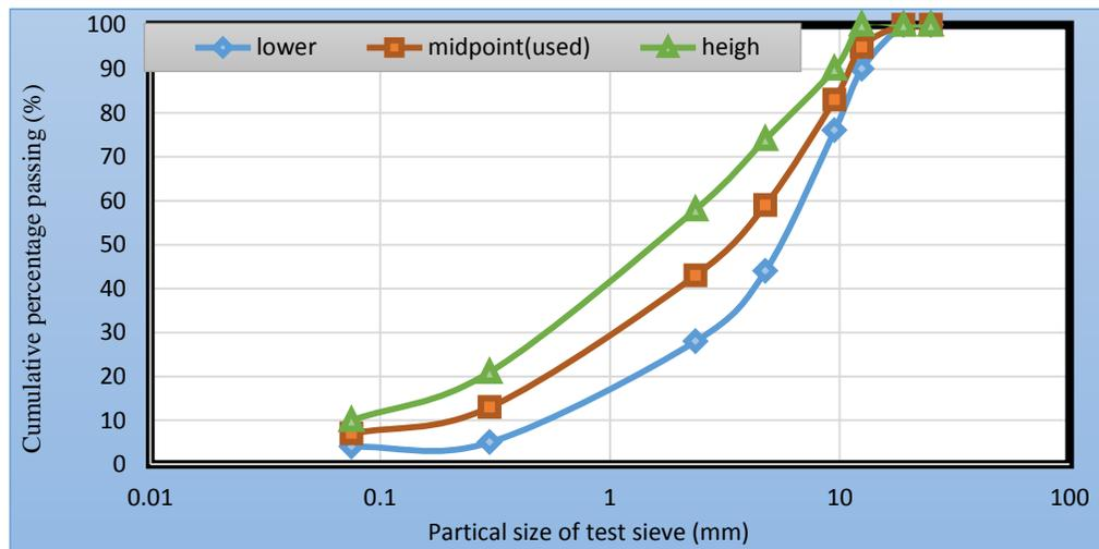
**Figure 1 Particle Size Distribution of the Used Gradation**
