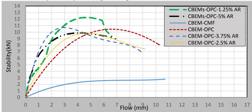
**Figure 4 Stability-Flow curves for CBEM comprised OPC and AR content compared with CBEMs-CMF**
