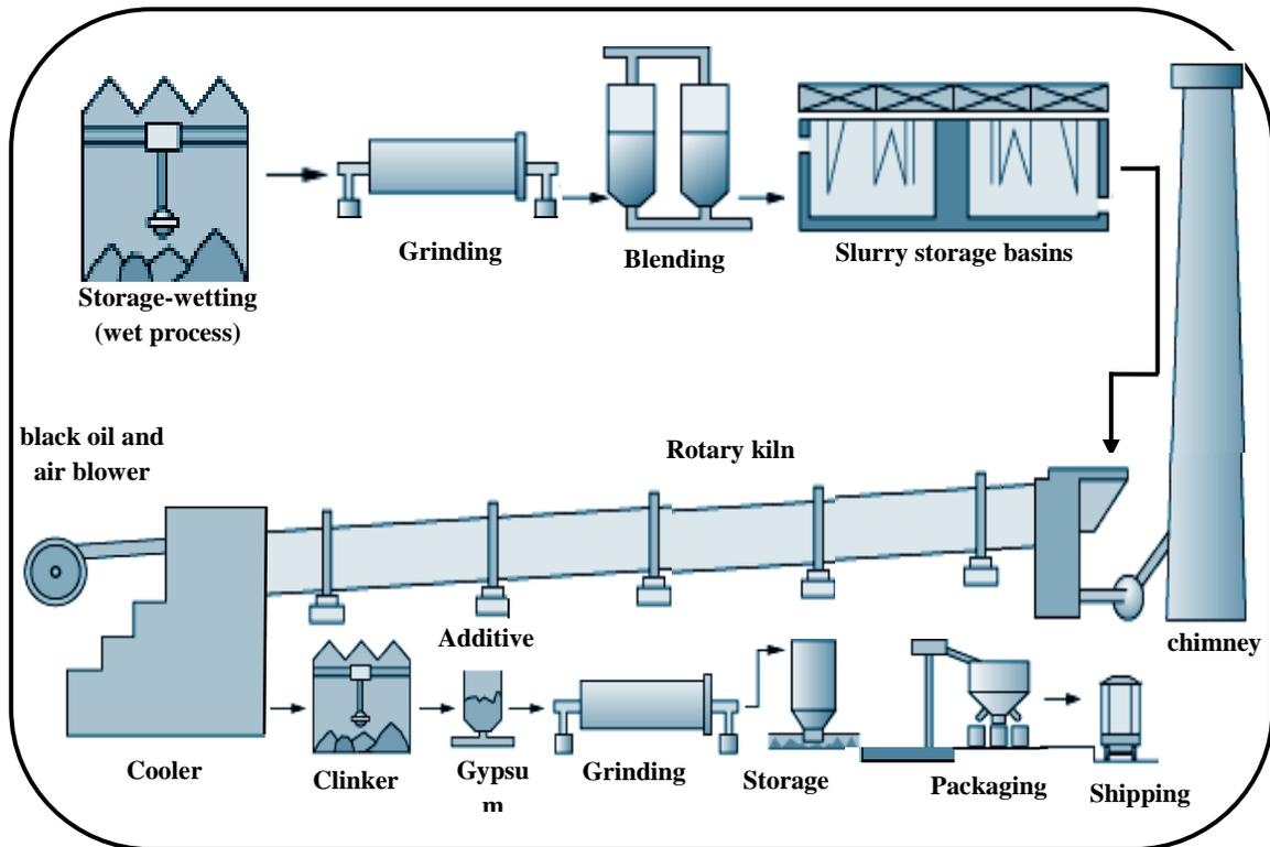
Figure (1) AL-kufa cement plant ( wet process)
