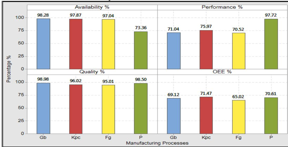
**Figure (2) Effect of Manufacturing Processes onto OEE Through January Month-2015**
