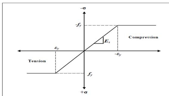
Figure (5) Stress-strain curve for steel reinforcement. Ref.[7]
