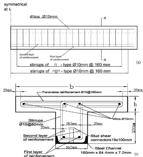
a) Reinforcement of concrete T-beam b) Section A-A
