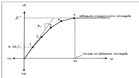
Figure (4) Simplified compressive uniaxial stress-strain curve for concrete. Ref.[5]
