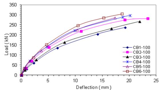
Figure (9) Variation of mid-span deflection with load (100% degree of shear connection)
