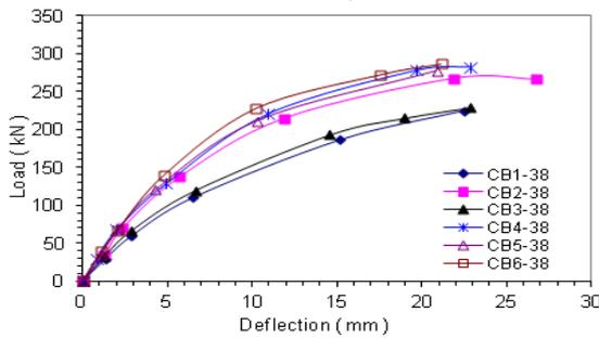
Figure (12) Variation of mid-span deflection with load (38% degree of shear connection)
