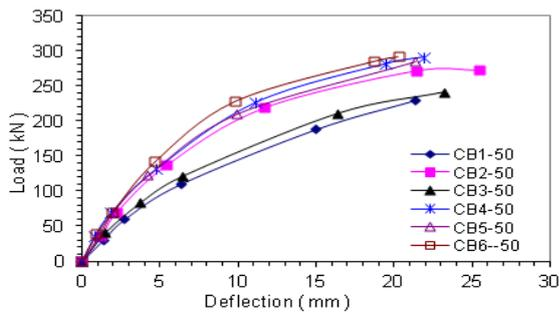
Figure (11) Variation of mid-span deflection with load (50% degree of shear connection)
