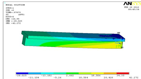
Figure (17) Stress variation in Z-direction along half span for beam TB1 at ultimate load
