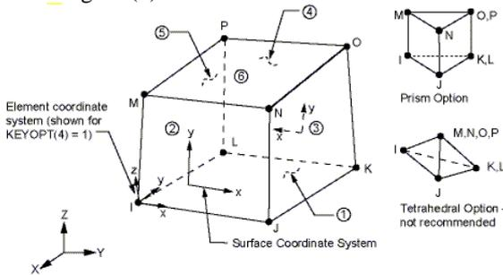
Figure (3) SOLID45 3D- Structural solid element. Ref.[3]
