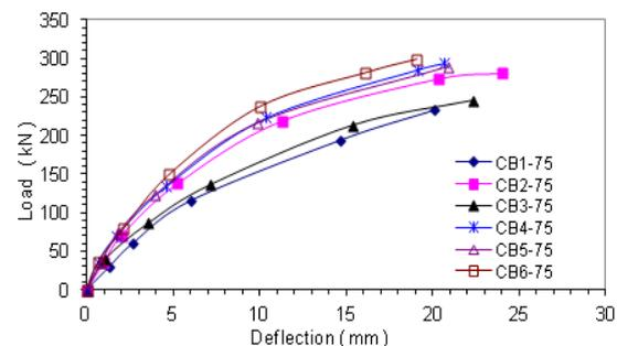
Figure (10) Variation of mid-span deflection with load (75% degree of shear connection)
