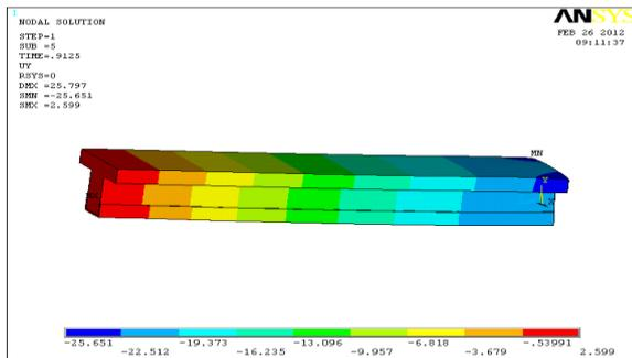
Figure (13) Deflection distribution along half span for beam CB1-38 at ultimate load
