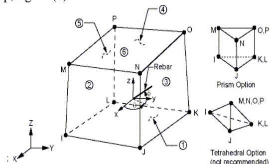
Figure (1) SOLID65 3D- Concrete element. Ref.[3]
