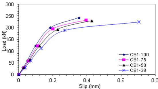
Figure (15) Variation of end-slip with load for beams CB1
