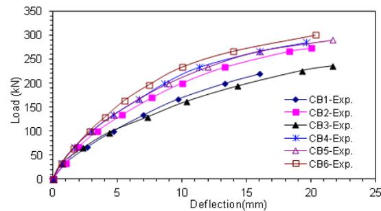
Figure (8) Variation of mid-span deflection with load (Experimental work). Ref.[6]
