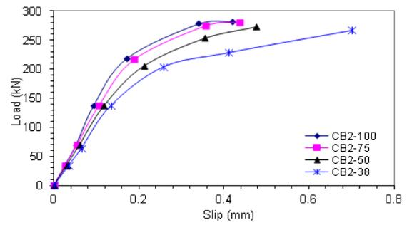
Figure (16) Variation of end-slip with load for beams CB2
