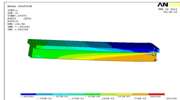
Figure (18) Strain variation in Z-direction along half span for beam TB1 at ultimate load
