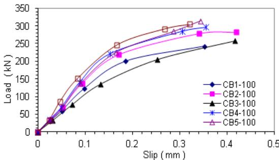
Figure (14) Variation of end-slip with load (100% degree of shear connection)
