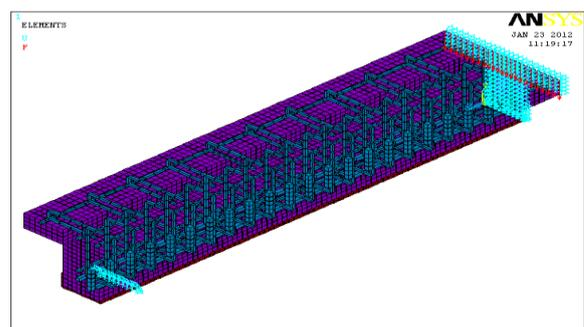
Figure (7) Representation of boundary conditions and applied loads (half span)
