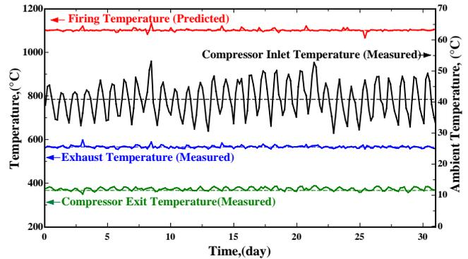
Fig. 4. Variation of operating temperatures of for Khor Al-Zubair GE unit during July 2016.
