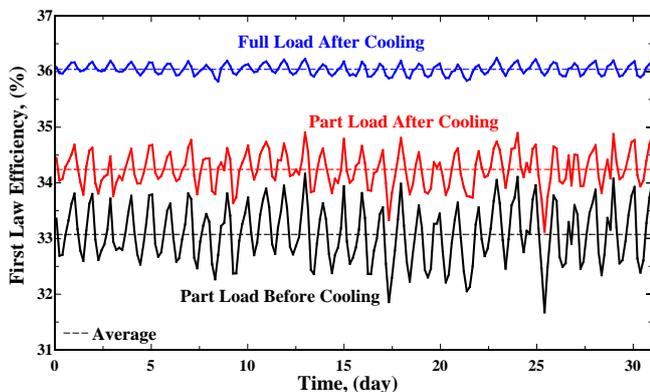
Fig. 6. Prediction of the first law efficiency of for Khor Al-Zubair GE unit before and after cooling with VCC.
