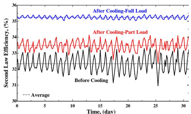
Fig. 9. Variation of second law efficiency of Khor Al-Zubair GE unit before and after cooling with VCC.
