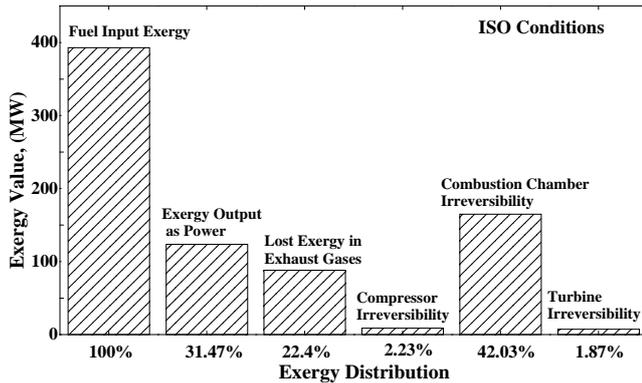
Fig. 3. Exergy (MW) distribution for Khor Al-Zubair GE unit at ISO conditions.
