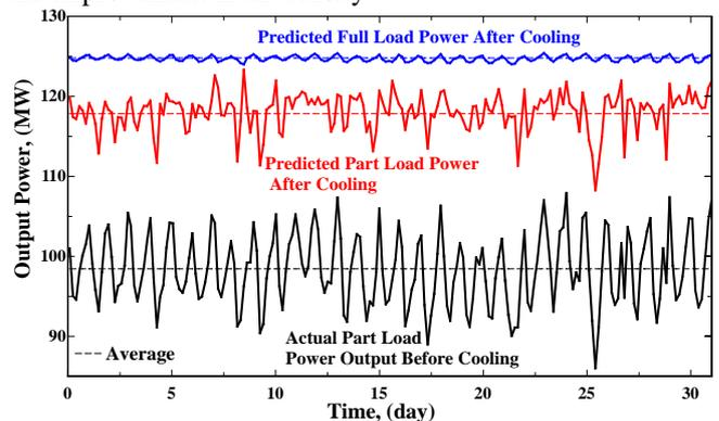
Fig. 5. Variation of power output from Khor Al-Zubair GE unit and power enhancement predicted after cooling with VCC.
