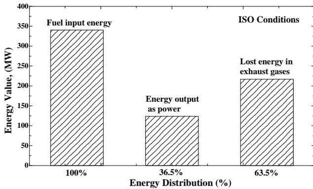
Fig. 2. Energy (MW) distribution for Khor Al-Zubair GE unit at ISO conditions.
