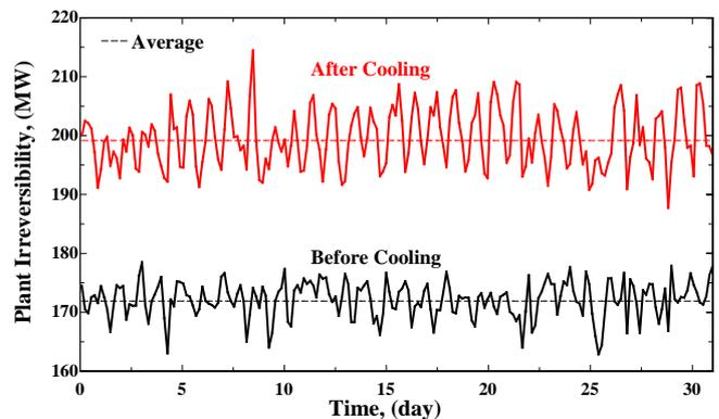
Fig. 8. Variation of total irreversibility of Khor Al-Zubair GE unit before and after cooling with VCC.
