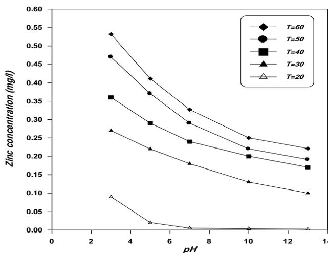
Fig.1: The relation between the pH and the zinc concentration for different temperature values at constant dose (15g), constant settling time (7 day)
