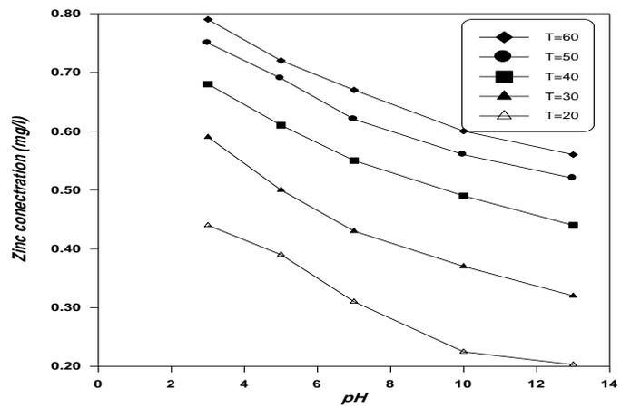
Fig. 5: The relation between the pH and the zinc concentration for different temperature values at constant dose (2.5g), constant settling time (7 day)
