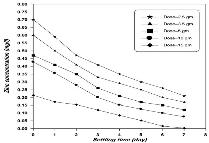
Fig.10: the relation between the settling time and the zinc concentration for different dose values at constant (pH=13), constant temperature (20C°)
