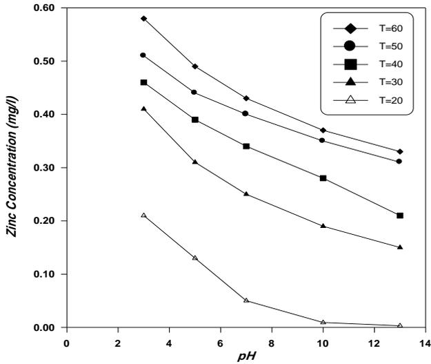
Fig. 2: The relation between the pH and the zinc concentration for different temperature values at constant dose (10g), constant settling time (7 day)
