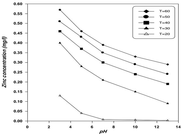
Fig. (3) The relation between the pH and the zinc concentration for different temperature values at constant dose (5g), constant settling time (7 day)
