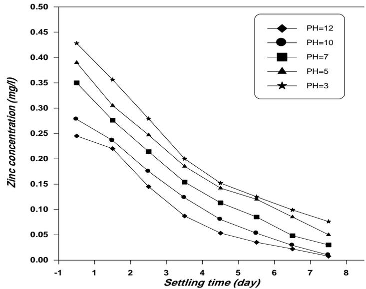
Fig.9: the relation between the settling time and the zinc concentration for different pH value at constant dose (10g), constant temperature (20 C°)
