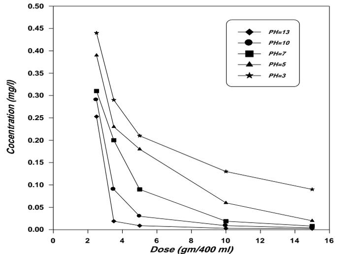
Fig.7: The relation between the dose and the zinc concentration for different PH values at constant temperature (T=20 oC), constant settling time (7 day)
