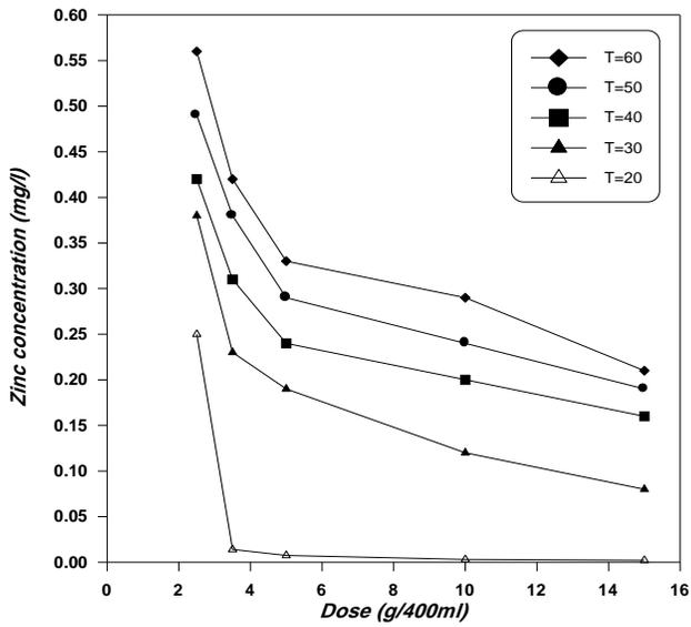
Fig.8: The relation between the dose and the zinc concentration for different temperature values at constant (pH=13), constant settling time (7 day)
