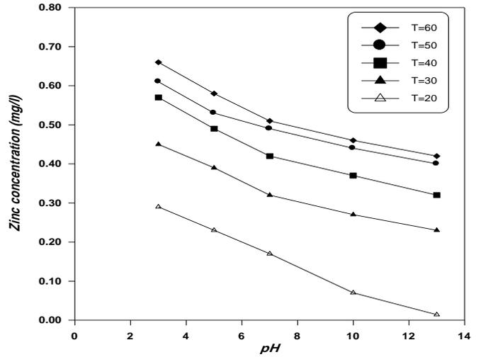
Fig. 4: The relation between the pH and the zinc concentration for different temperature values at constant dose (3.5g), constant settling time (7 day)
