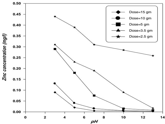
Fig.6: the relation between the pH and the zinc concentration for different dose at constant temperature (T=20), constant settling time (7 day)
