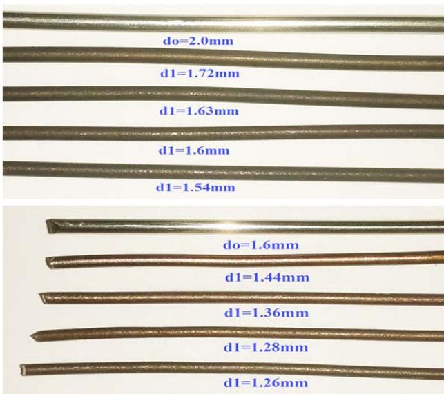
Fig. 7: Photos of passed wires produced by present DLD machine.
