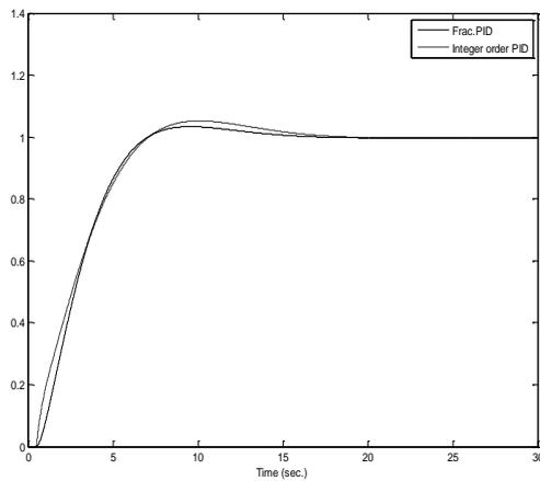
Fig. 3 step response for SOPDT.
