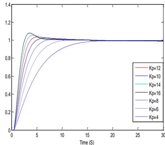
Fig. 7 step response for FOPDT for different values of  $K_p$  with FOPI controller.
