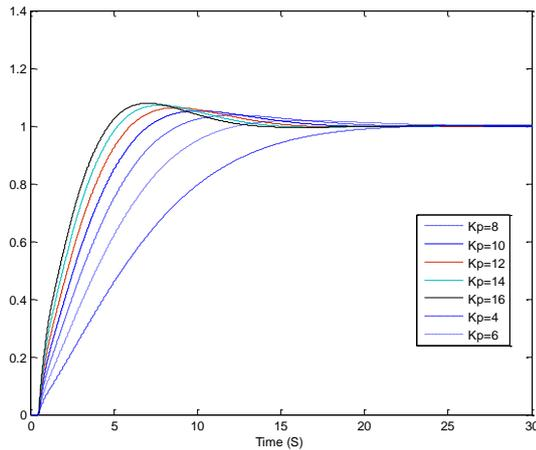
Fig. 8 step response for SOPDT for different values of  $K_p$  with IOPID controller.
