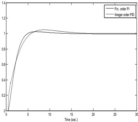
Fig. 2 step response for FOPDT.
