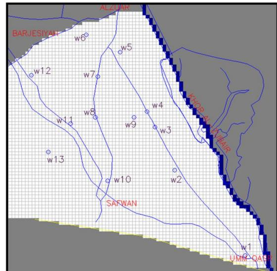
Fig. 4 Layout of monitoring wells on MODFLOW model grid.
