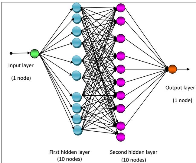
Fig. 5 Configuration of ANN with input layer of one node and two Hidden layers, each of ten nodes
