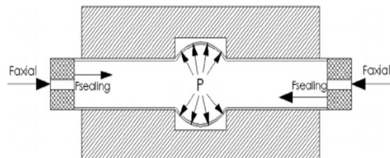
Fig. 1 Tube hydroforming process.
