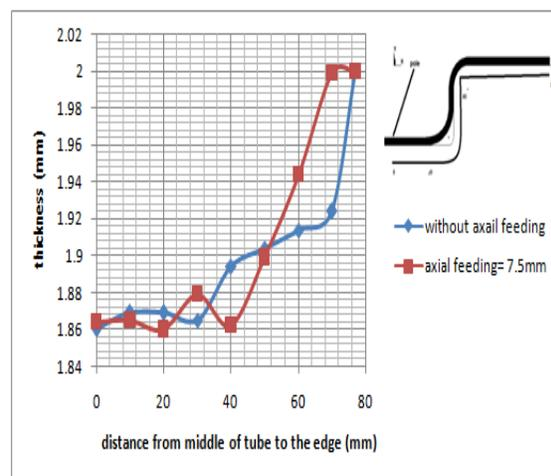
Fig. 7 The variations in thickness on the tube wall from middle tube to the edge, for two cases ( without axial feeding and with axial feeding value (7.5mm).
