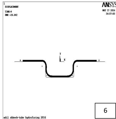
Fig. 4 Different stages of material deformation during simulation in tube hydroforming process.
