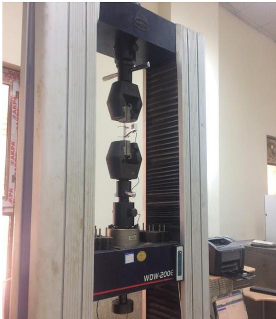
Fig. 3 The tensile test machine used.
