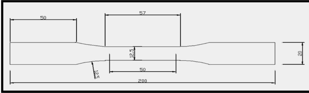
Fig. 2 The dimensions of the tensile test specimen according to ASTM standard E8M specification.
