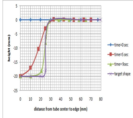
Fig. 9 Shape conformation of the tube from center to the edge throughout the forming process.
