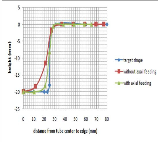
Fig. 8 Shape conformation of the final tube from center to the edge after forming process.
