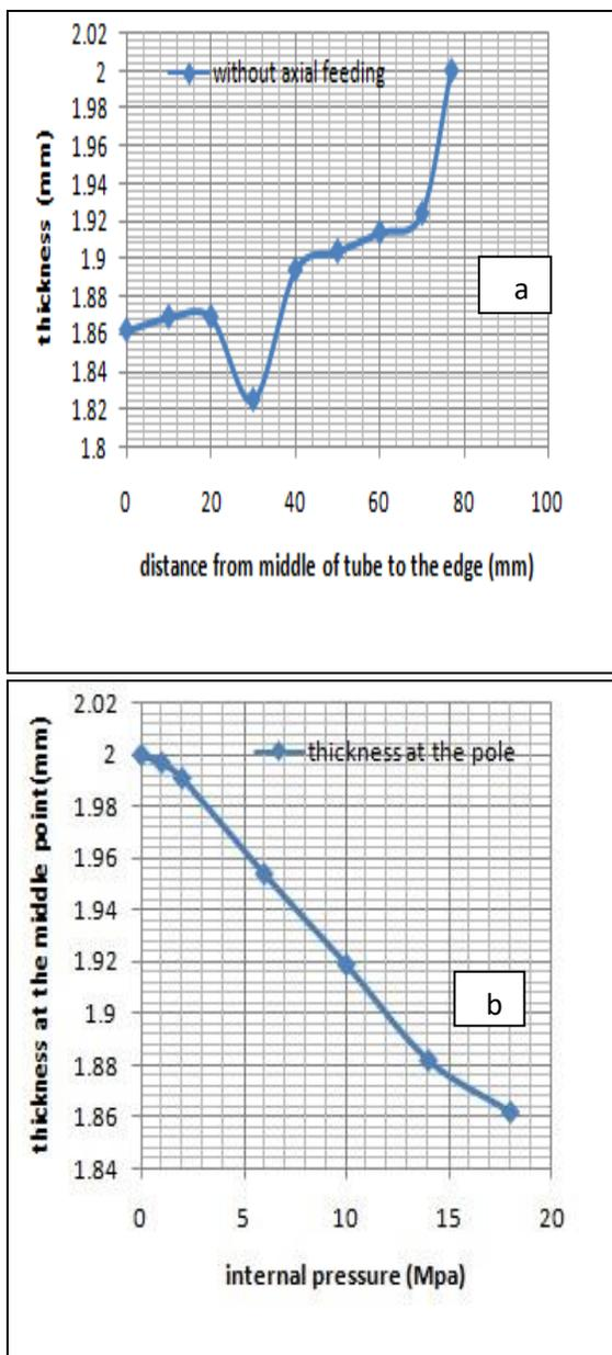
Fig. 6 The thickness distribution on the tube wall. 6a, thickness distribution from middle to the edge tube. 6b, variation in the pole thickness during the hydroforming process.
