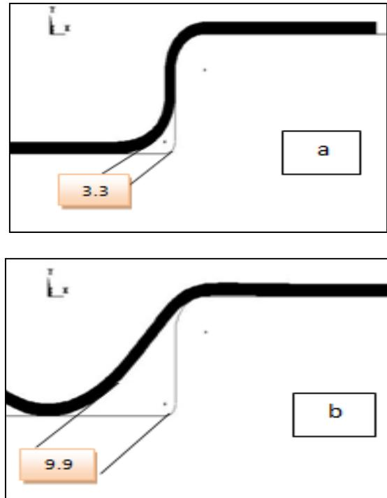
Fig. 10 Shape conformation of the final tube at corner radius (a) with axial feeding, (b) without axial feeding.
