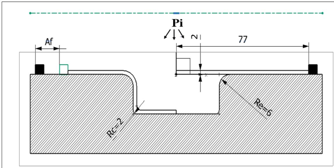
Fig. 5 Representation of the tube hydroforming process .
