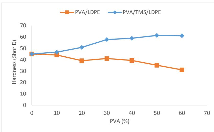
**Fig.4: Hardness of PVA/LDPE with and without silane.**
