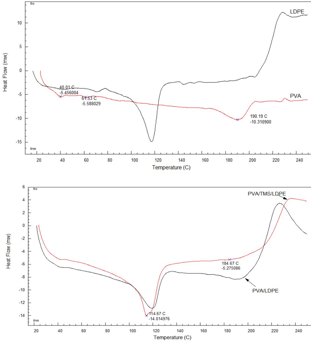
**Fig.9: DSC curves for: LDPE, PVA, PVA/LDPE, d)PVA/TMS/LDPE**
