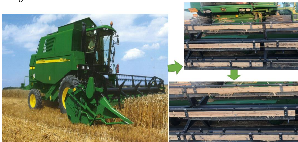
Figure (2): Reel with rubber strips for John Deere wheat combine harvester model 1450 CWS
