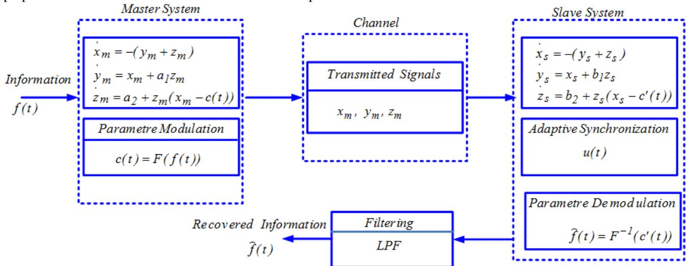
Fig. 8 The communication scheme based on adaptive synchronization of the chaotic Rössler systems.
