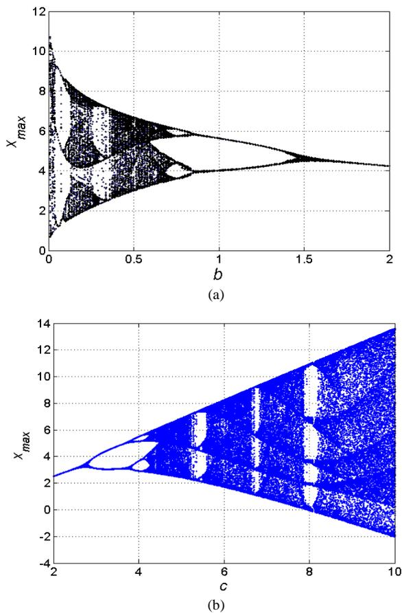
Fig. 1 The bifurcation diagram of Rössler system for  $a = 0.2$ .
