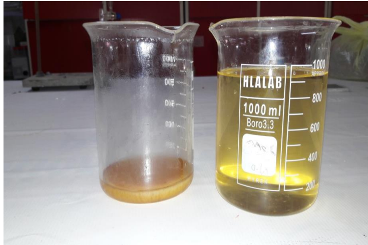
Fig (2) The Schemes of Synthesized Biodiesel and glycerin
