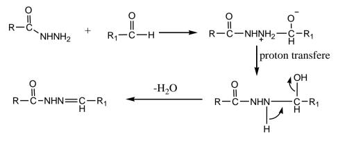
The IR spectra of compounds (15-18), (Table 4), showed absorption bands at (1689-1655)  $Cm^{-1}$  for the hydrazide C=O bond stretching and at (1636-1604)  $Cm^{-1}$  for the imino C=N bond stretching.
