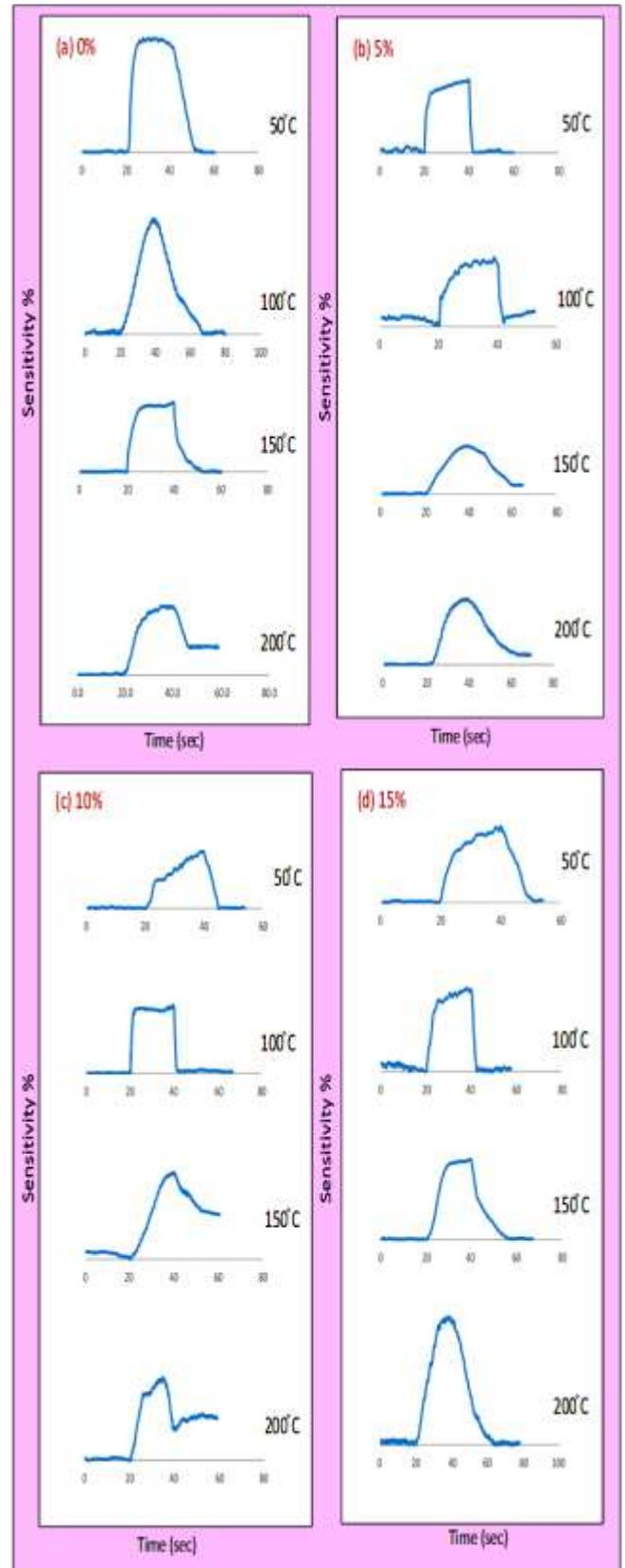
Fig. 4: Response of In<sub>2</sub>O<sub>3</sub> – Ag<sub>x</sub>O thin films deposited on porous silicon substrate toward 400 ppm NH<sub>3</sub> gas.
