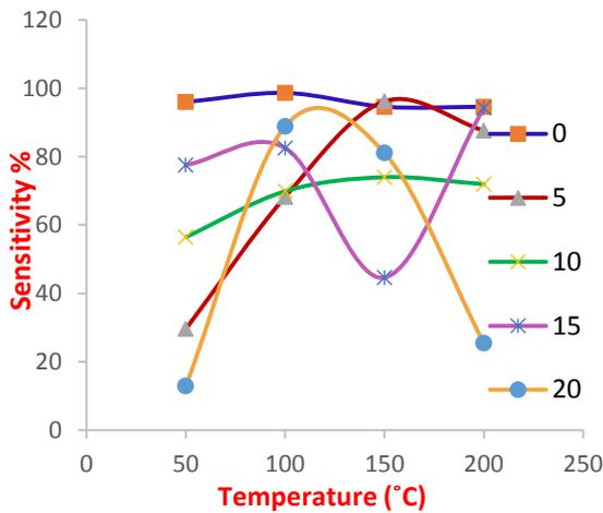
Fig. 5: Sensitivity versus temperature for In<sub>2</sub>O<sub>3</sub> – Ag<sub>x</sub>O sensors at different Ag<sub>x</sub>O concentration on porous silicon.
