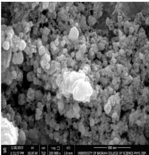
Fig. 3: FE-SEM images of  $\text{In}_2\text{O}_3 - \text{Ag}_x\text{O}$  thin films at 15% mixed ratio on porous silicon substrate.
