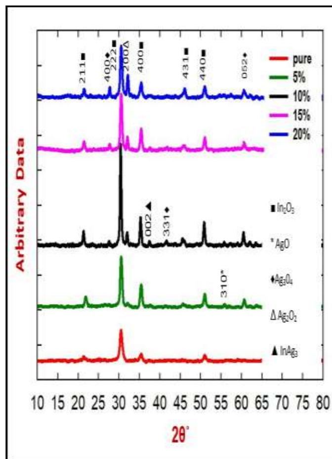
Fig. 1: The XRD patterns of mixed  $\text{In}_2\text{O}_3$  –  $\text{Ag}_x\text{O}$  thin films deposition on glass substrate.
