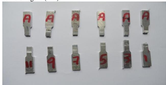
Fig.11 Tensile Test Specimen after testing
