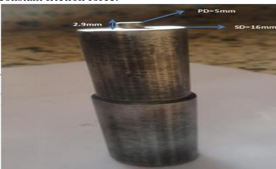
Fig.4 Tool for FSW and FSP
