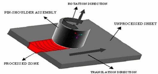
Fig.1 Schematic of friction stir processing (FSP) [ 5 ]
