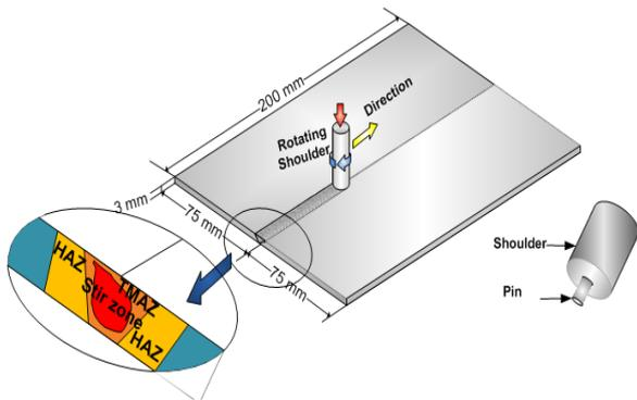
Fig.2 6061-T6 AA plates dimensions and Schematic of friction stir welding (FSW)
