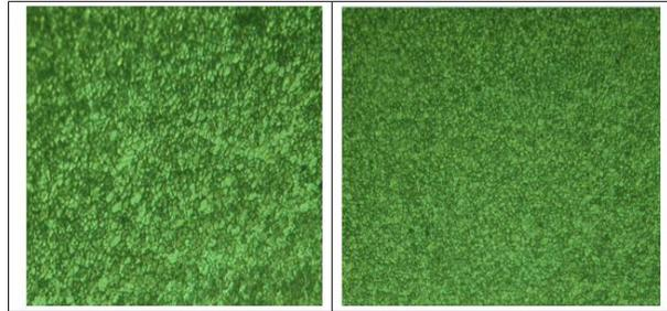
Nuggetzone for FSW at 1300rpm,60m Nuggetzone for FSP at 1300rpm,60mm/min
