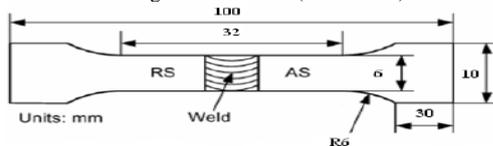
Fig.7 standard tensile specimen
