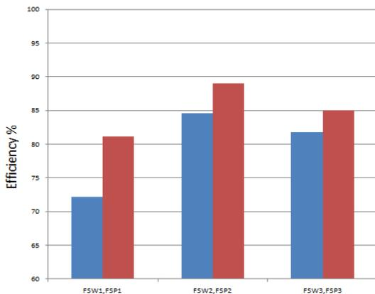
Fig.13 results of efficiency for tensile test
