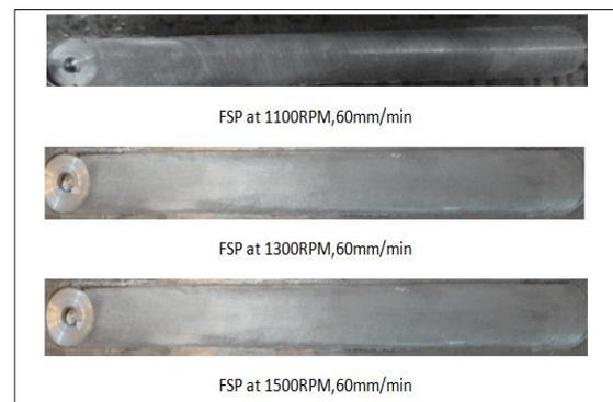
Fig.10 The appearance of upper surface of welding beads of 6061-T6 AA plates produced by FSP.
