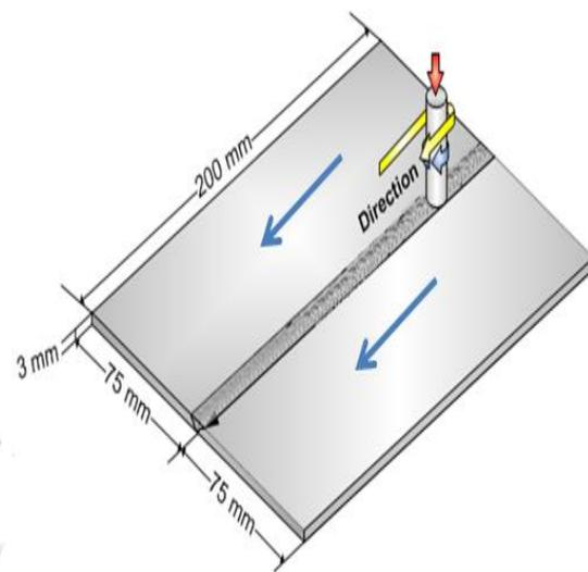
Fig.5 FSP process for 6061 – T6 plates
