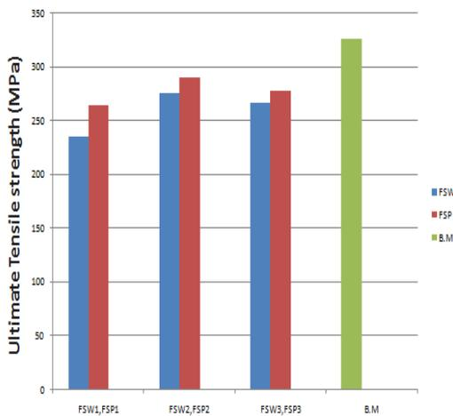
Fig.12 Tensile test results
