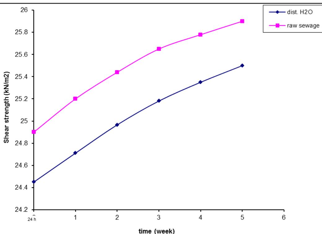
**Fig. (5) Shear strength - time relationship of soil with distilled water and raw sewage as pore fluid**
