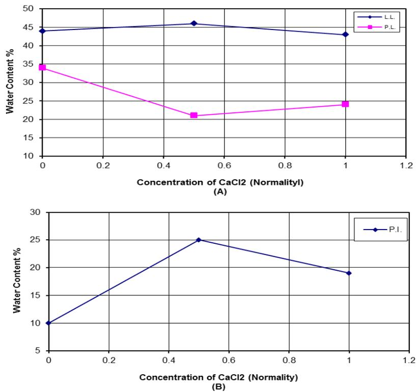
**Fig (3) Effect of Calcium Chloride on Atterberg Limits**
