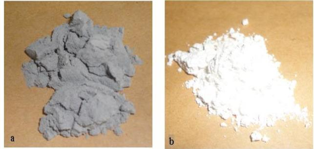
Fig. 1 The photographs of (a) the Al fine powder, and (b) ZrO<sub>2</sub> .
