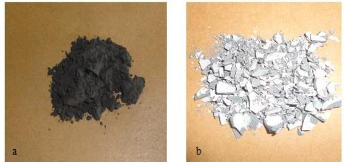
Fig. 3 The photographs of the (a) ZrO<sub>2</sub>-Cu coating powder succeeded after extraction from filter and milling ,sieved it below 63μm (b) ZrO<sub>2</sub>-Cu coating powder failed.
