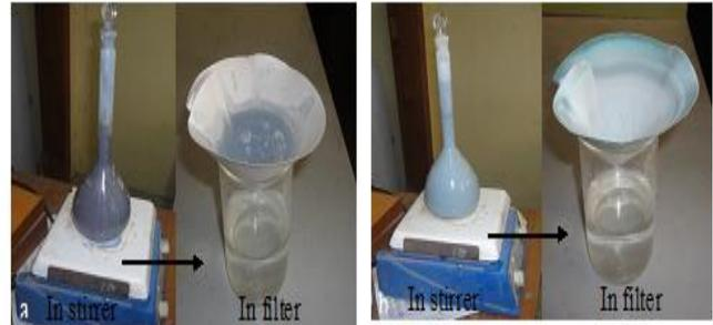
Fig. 2 The photographs of the (a) ZrO<sub>2</sub>-Cu coating powder succeeded on stirrer plate and filter, (b) ZrO<sub>2</sub>-Cu coating powder failure on stirrer plate and filter.
