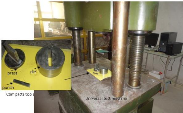
Fig. 5 Computer controlling versatile electronic testing machine and the compaction tools.
