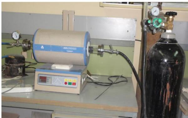
Fig. 6 Vacuum tube furnace.
