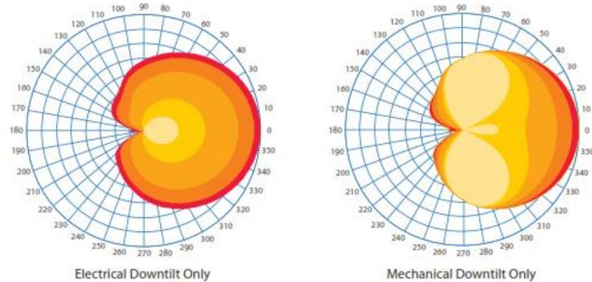
**Figure (3):** Electrical versus mechanical down tilt angle comparison
