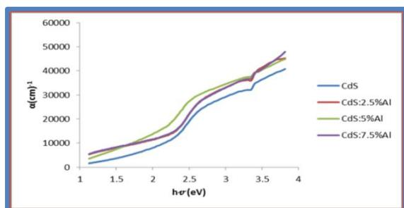
**Fig5: Absorption coefficient of CdS and CdS:(2.5,5,7.5)%Al**
