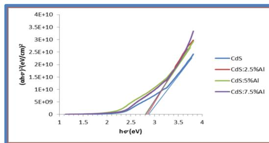
**Fig 6: The Energy Gap for the Allowed Direct Transition  $(\alpha h\nu)^2$  as a Function of Photon Energy CdS and CdS:(2.5,5,7.5)%Al**
