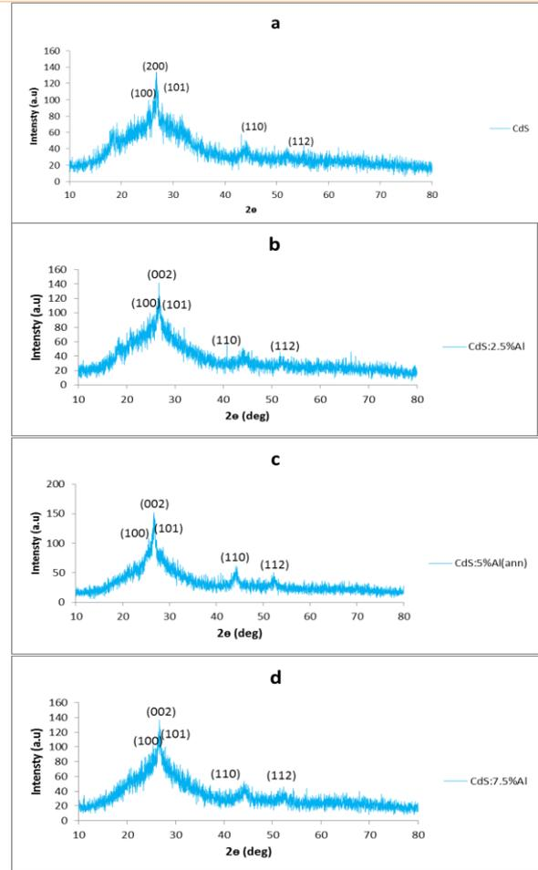
**Fig1: XRD pattern of deposited CdS:Al for a:CdS b:CdS:2.5%Al c:CdS: 5%Al d:CdS:7.5%Al**
