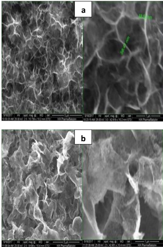
**Fig2. SEM images of a: CdS b: CdS:7.5%Al**
