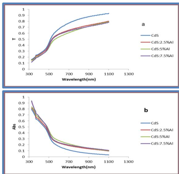
**Fig4. a optical transmittance and b theoptical absorption curves of CdS and CdS:(2.5,5,7.5)%Al**
