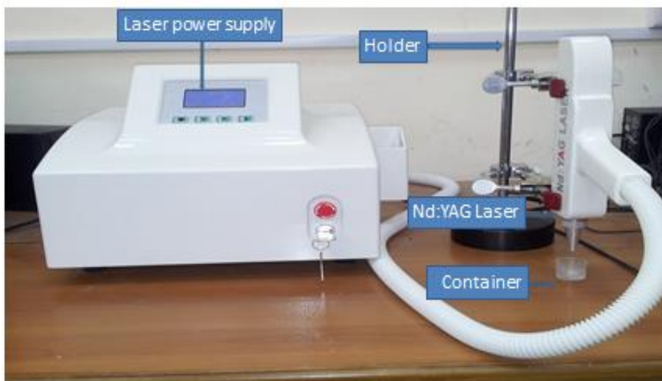
Figure 1: The experimental setup of the laser ablation process.
