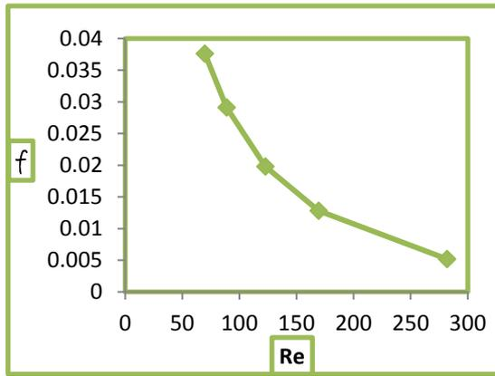
Figure (11). Friction Factor versus Reynolds Number (propylene glycol)
