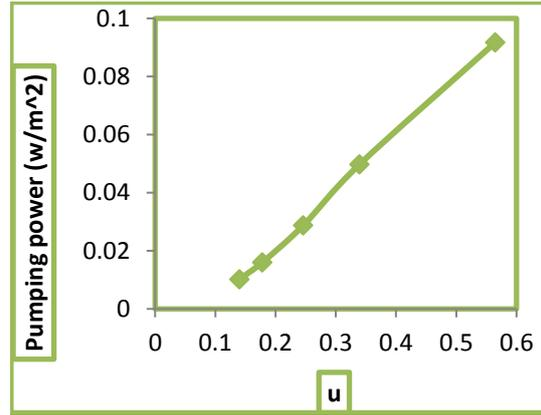
Figure (12). Pumping Power versus Fluid Velocity
