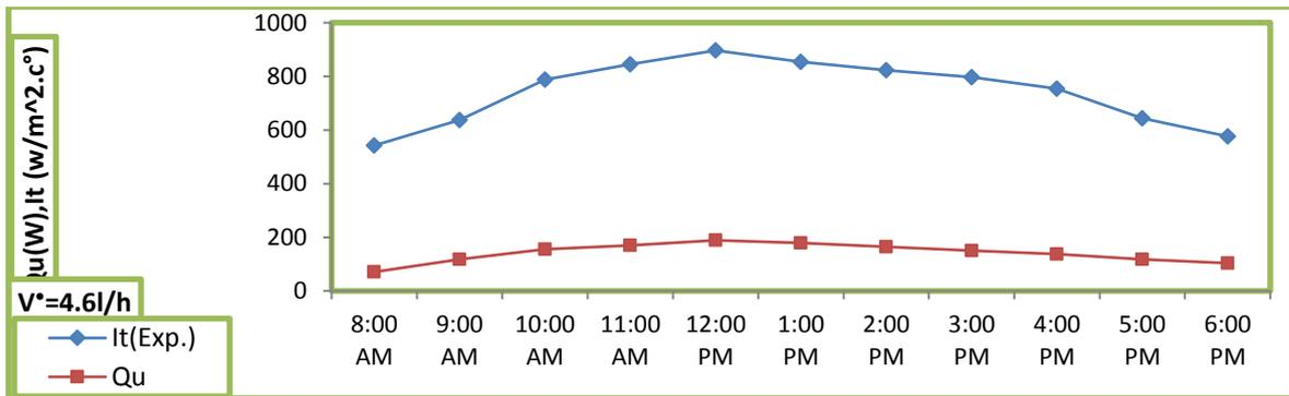
Figure (8). Useful Energy and Solar Radiation with Time at ( $T_{f(in)} = 15^{\circ}\text{C}$ ).
