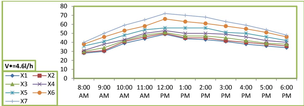
Figure (5b) Temperatures Distribution of Absorber Plate with Time ( $T_{f(in)} = 20^{\circ}\text{C}$ ).
