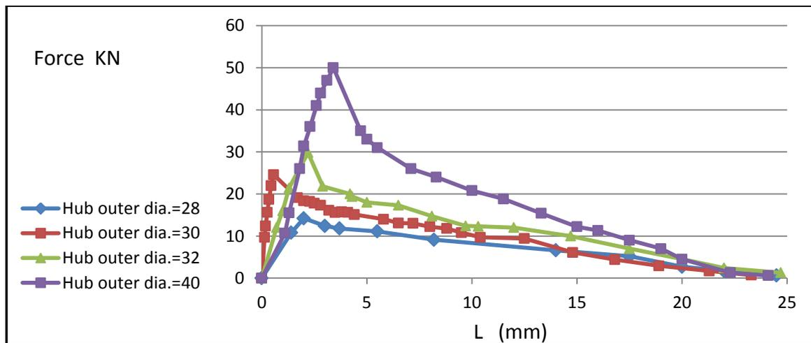
**Figure5:** Decoupling different hub thickness
