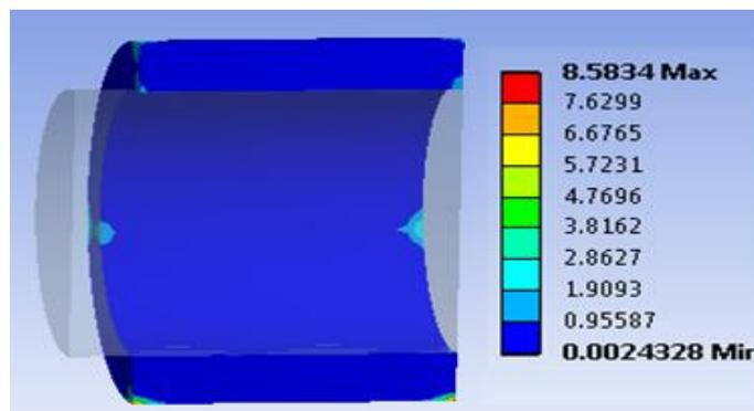
**Figure 9:**Equivalent stresses after coupling for hub with outer diameter 30 mm
