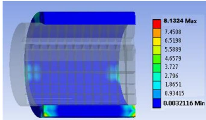
**Figure 10:** Equivalent stresses after coupling for hub with outer diameter 28 mm
