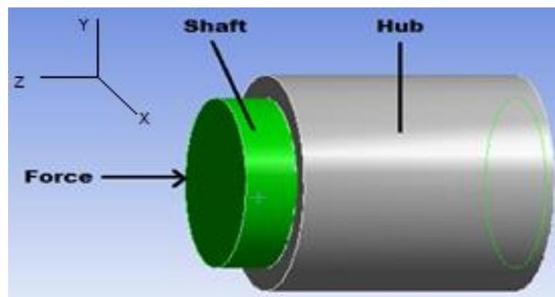
**Figure 6:** Schematic diagram of the interference fit
