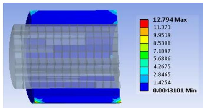
**Figure 8:** Equivalent stresses after coupling for hub with outer diameter 32 mm
