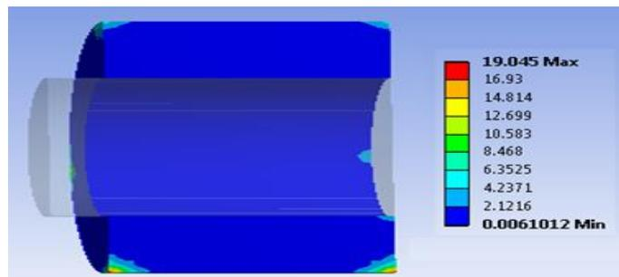
**Figure 7:** Equivalent stresses after coupling for hub with outer diameter 40 mm
