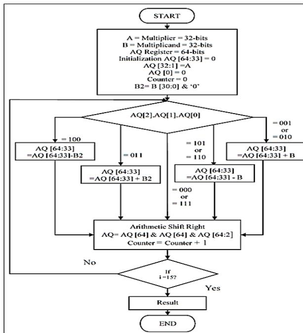
Figure 15: Flowchart of the modified Booth's algorithm
