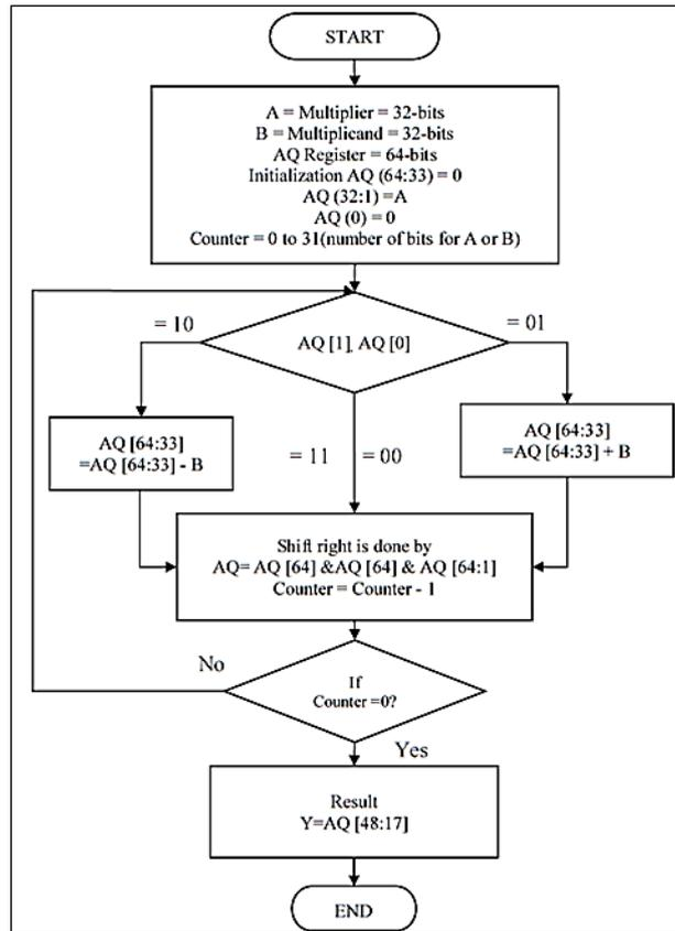
Figure 13: Flowchart of the Booth's multiplier using VHDL
