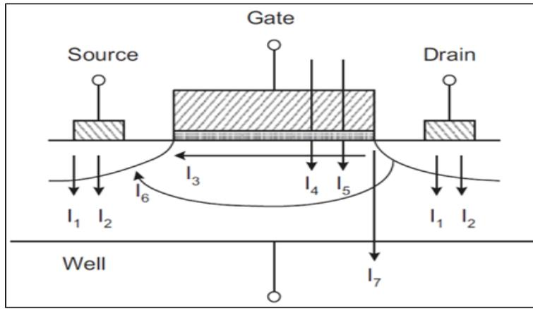
Figure 1: Sources of Static Power Dissipation [16]
