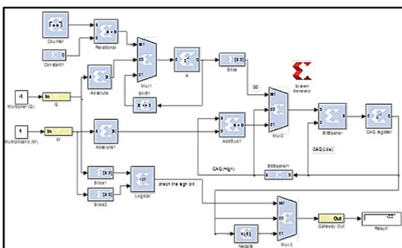
**Figure 5:** The Proposed Sequential Multiplier Using XSG Blocks
