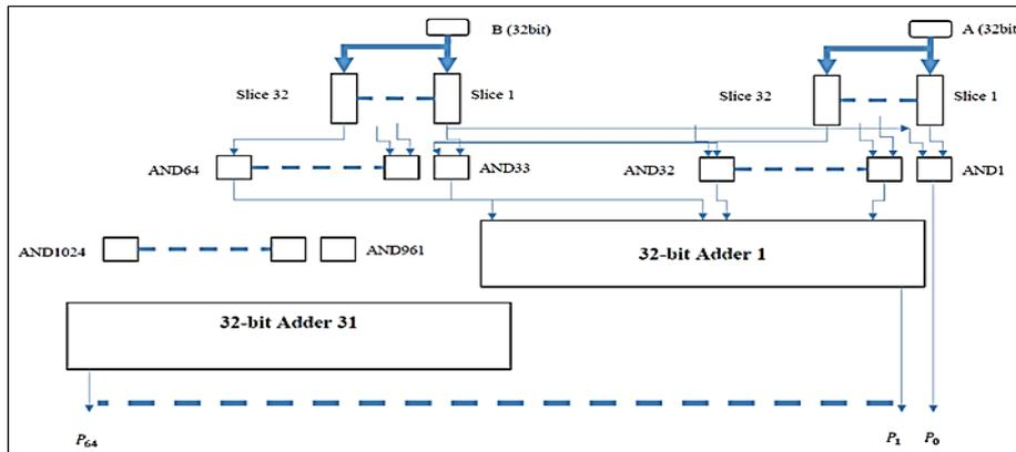
Figure 10: Subsystem of 32x32 bit array multiplier
