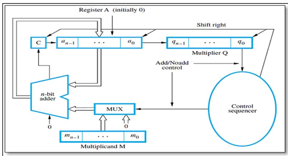
Figure 2: Hardware implementation of the sequential multiplier [28]
