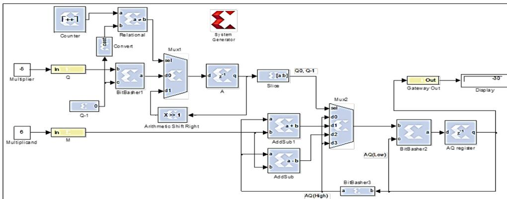
Figure 11: Proposed Booth's multiplier using XSG blocks
