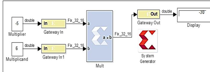
Figure 8: Proposed design using Xilinx LogiCORE™ IP Multiplier
