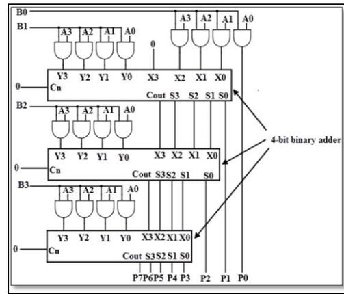
Figure 4: Array Multiplier 4-bit x 4-bit implementation [31]
