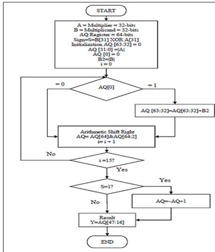
Figure 7: Flow chart of the proposed sequential multiplier
