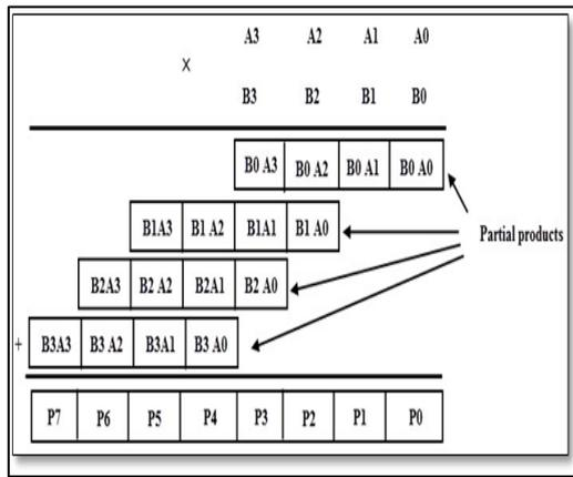
Figure 3: Array Multiplier 4-bit x 4-bit algorithm [30]
