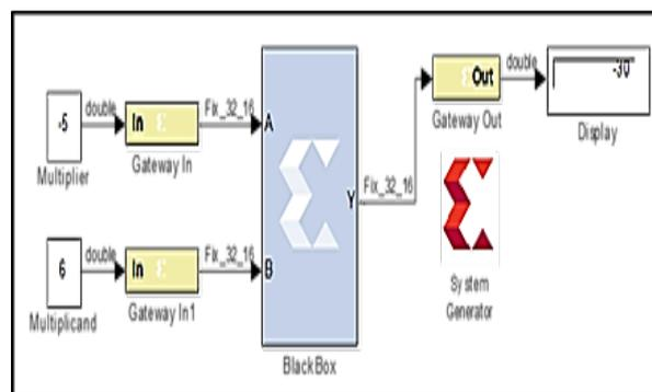
**Figure 6:** Proposed design of Sequential Multiplier using VHDL code
