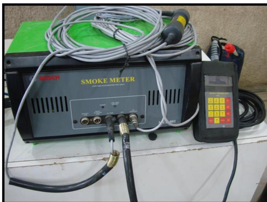
**Plate (6): The BOSCH Smoke Meter with the Remote Control**
