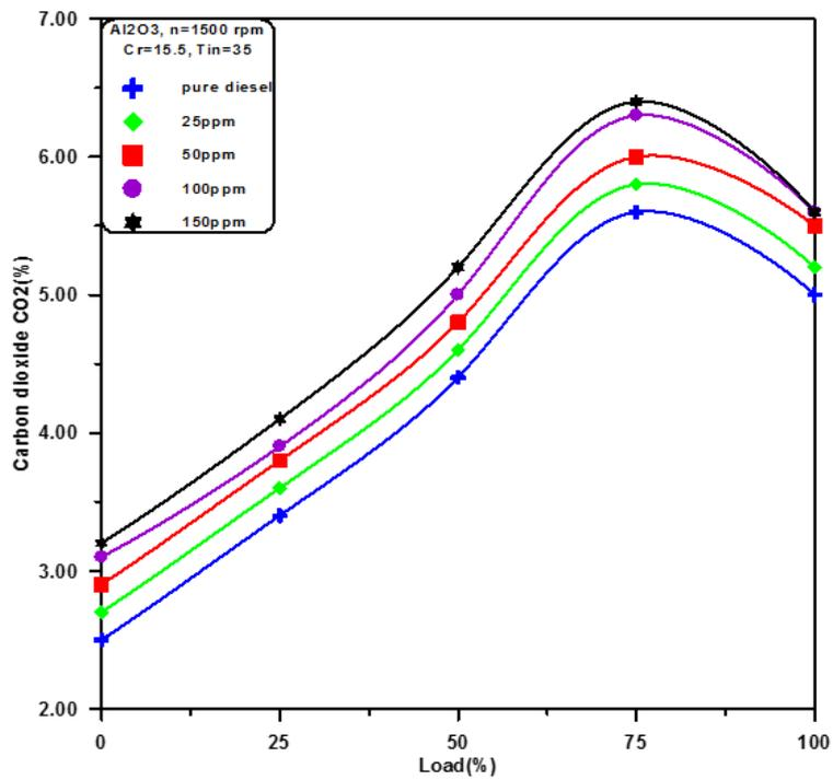
Figure 4 Variation of Carbon Dioxide with Load
