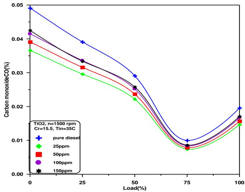
Figure 3 Variation of Carbon Monoxide with Loads
