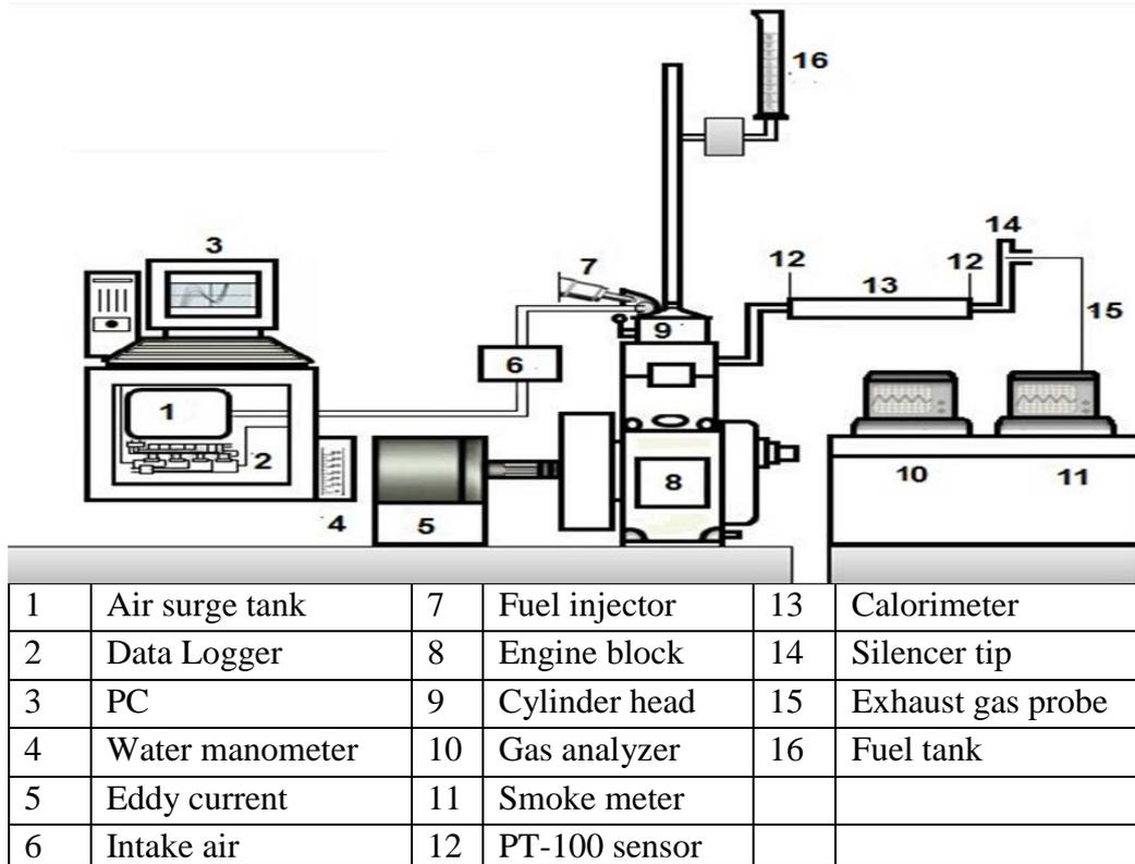
Fig (1) Schematic Diagram of Experimental Set Up.
