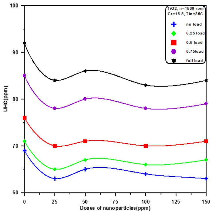
**Fig 11: Variation of Unburnt Hydrocarbon Emissions with Respect To Nanoparticles Dose Level.**
