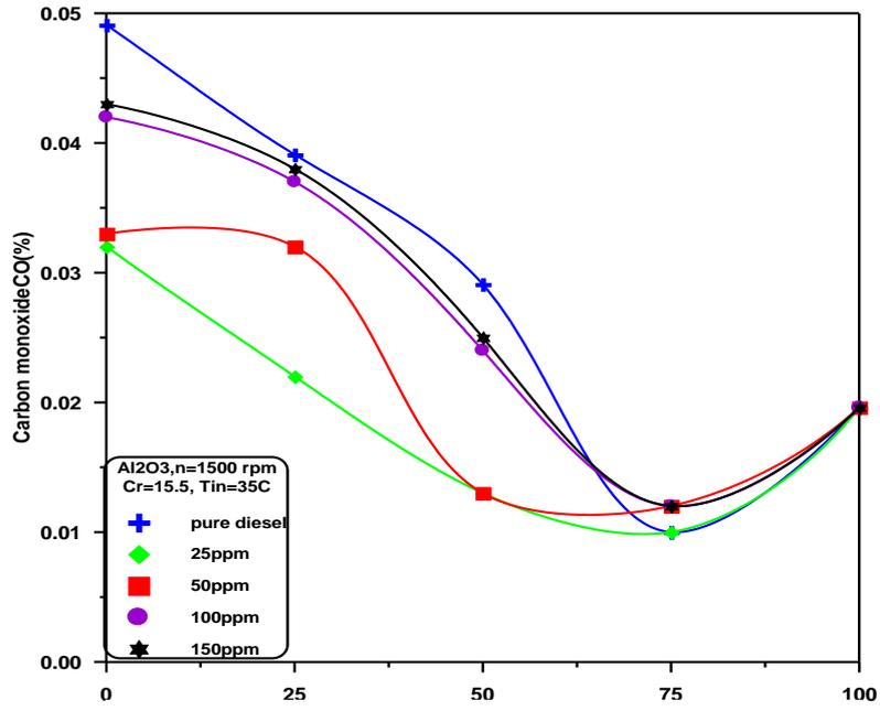
Figure 2 Variation of Carbon Monoxide with Loads
