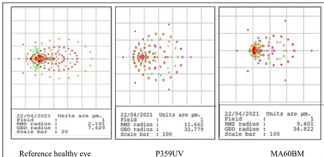
Figure 4: Polychromatic spot diagram for models' eye with refractive IOLs implanted
