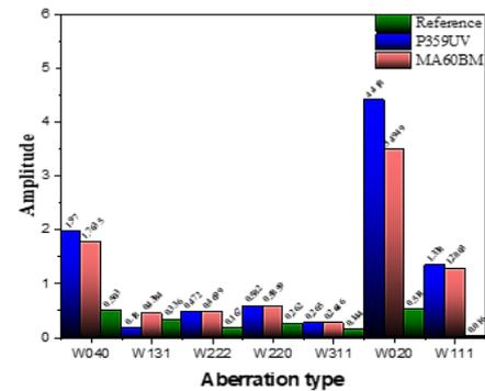
**Figure 6:** monochromatic aberration of (LBEM) and refractive IOL
