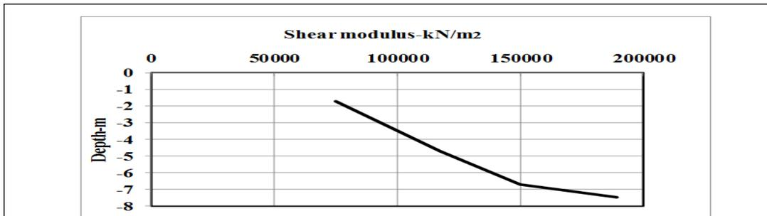
**Figure 17: Variation of shear modulus with depth for site HP under Iraqi earthquake of amplitude 0.05g.**
