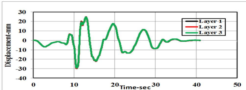
Figure 20: Displacement – time history for site H8, under Iraqi earthquake of amplitude 0.05g.
