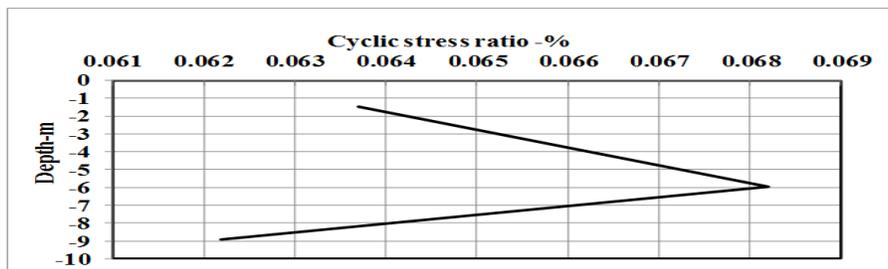
**Figure 29: Variation of cyclic stress ratio with depth for site H8, under Iraqi earthquake of amplitude 0.05g.**
