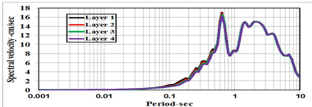
**Figure 12: Spectral velocity– period to response spectra with (5% damping) for site HP under Iraqi earthquake of amplitude 0.05g.**
