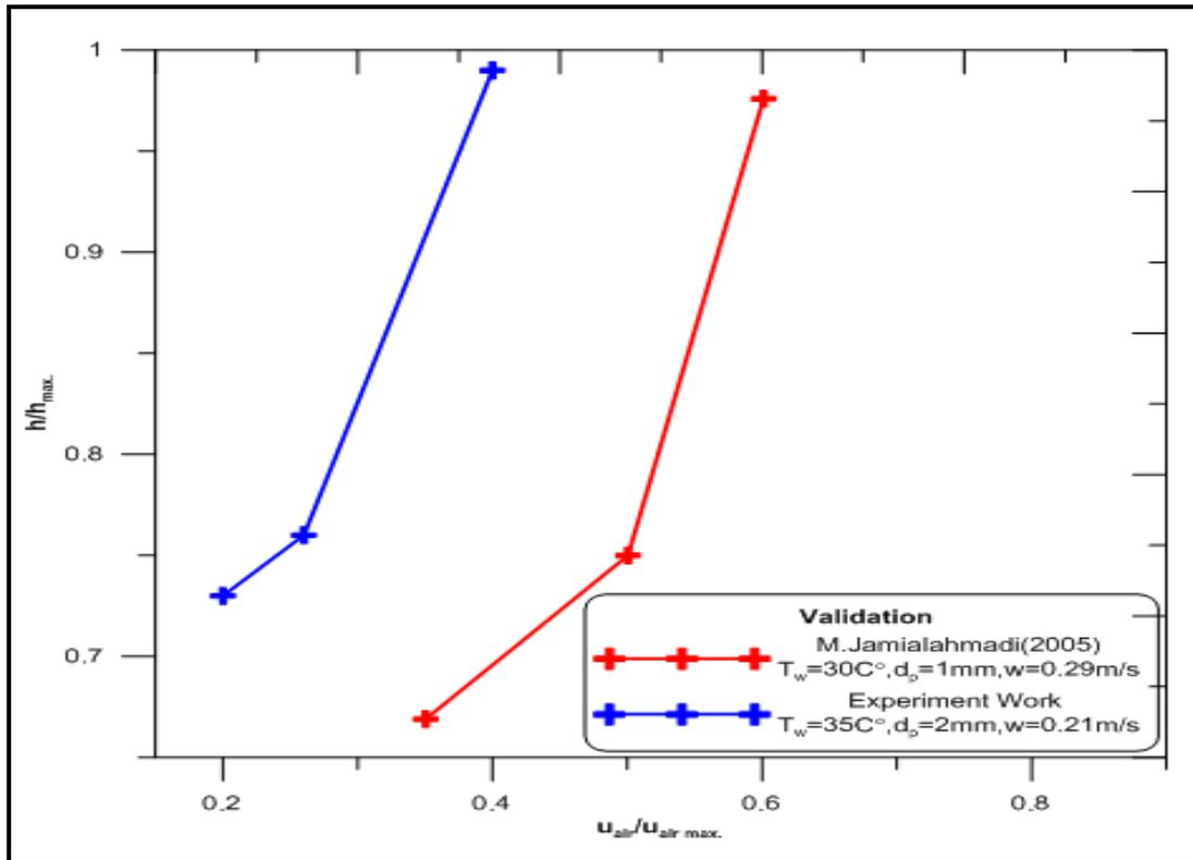
Figure (5): Comparison heat transfer coefficient with [15] versus uair (m/s).
