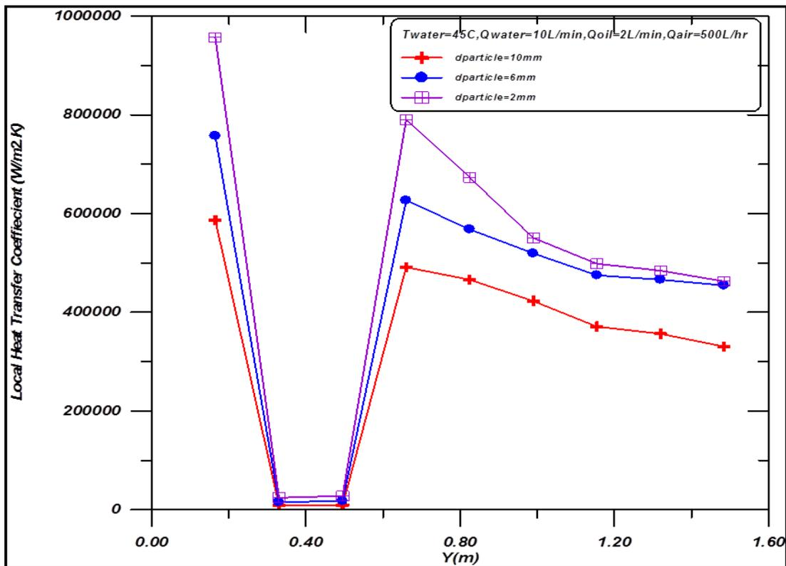
Figure (4): Coefficient heat transfer along pipe.
