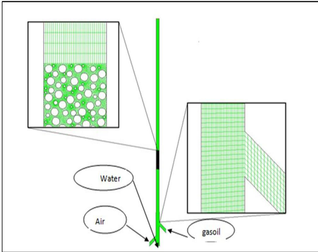
Figure (2): Geometry and Mesh of modeler.
