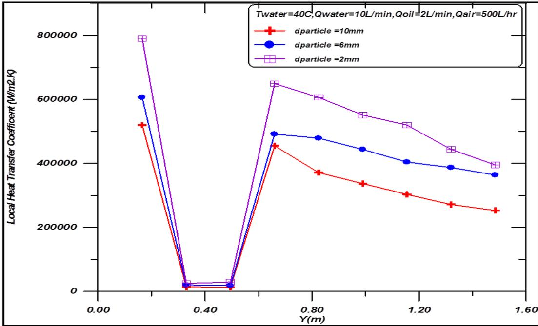
Figure (3): Heat transfer Coefficient along pipe.
