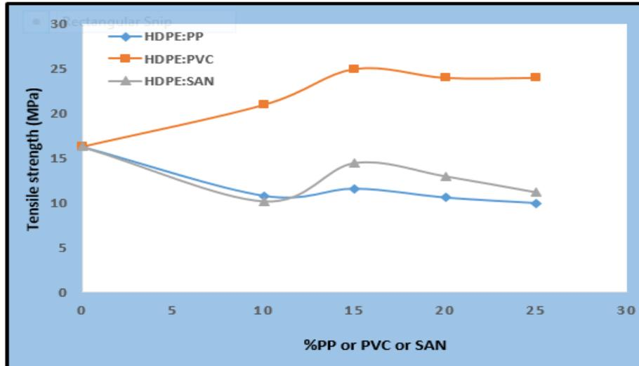
**Fig. (4): Tensile strength for binary polymer blends (PE: PP), (PE: SAN) and (PE: PVC) as a function of second materials [(PP), (SAN) or (PVC)] content in blend.**
