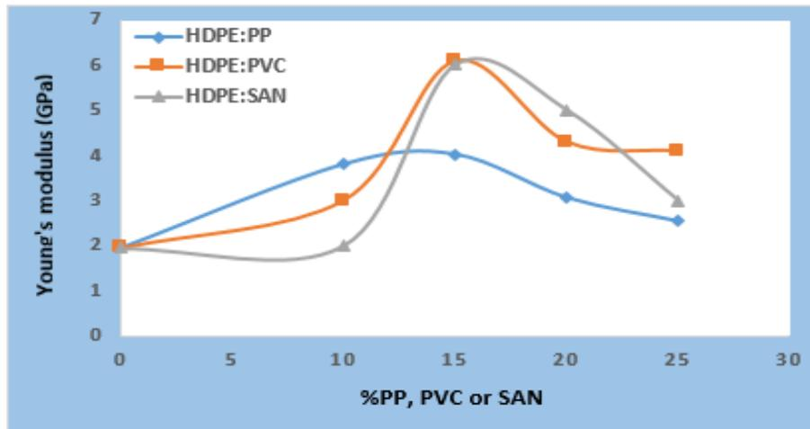
Fig. (5): Young's modulus for binary polymer blends (PE: PP), (PE: SAN) and (PE: PVC) as a function of second materials [(PP), (SAN) or (PVC)] content in blend.
