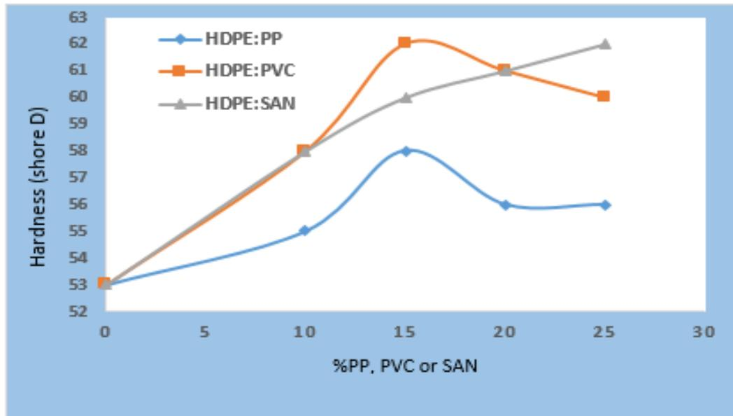
**Fig. (7): Hardness for binary polymer blends (PE: PP), (PE: SAN) and (PE: PVC) as a function of second materials [(PP), (SAN) or (PVC)] content in blend.**
