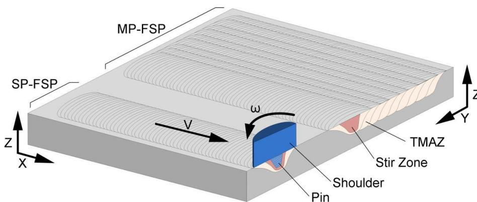
**Fig. (1): Schematic diagram of FSP process (Alberto *et.al.*, 2017).**
