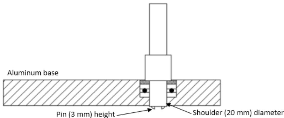
**Fig. (3): Schematic diagram of shoe tool**
