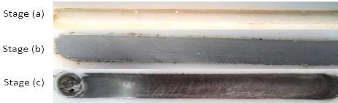
**Fig. (2): Illustrated three stages of FSP technique.**
