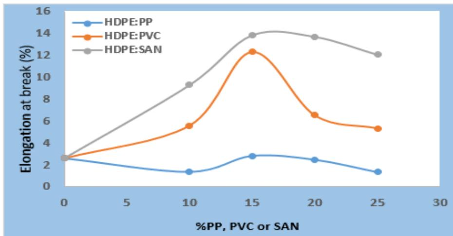
Fig. (6): Elongation at break for binary polymer blends (PE: PP), (PE: SAN) and (PE: PVC) as a function of second materials [(PP), (SAN) or (PVC)] content in blend.
