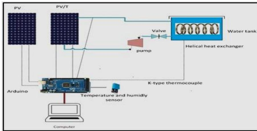
Figure 2: Schematic diagram of proposed PVT arrangement
