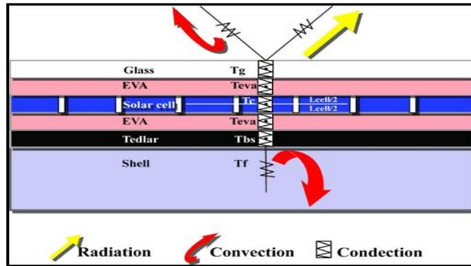
Figure 1: Heat transfer modes and equivalent thermal network
