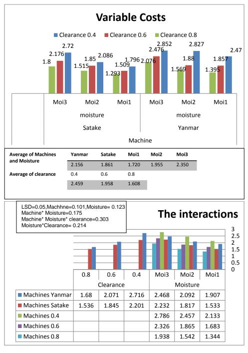
Fig (2) IIIustartes the Effect of Machines Types, Clearance and Grain Moisture on the Variable Costs \$\Ton.
