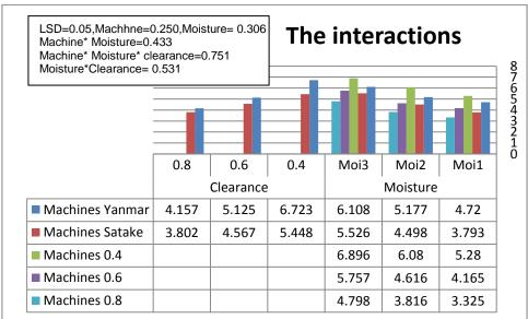
Fig (3) IIIustartes Effect of Machines types , Clearance and Grain Moisture on the Total Costs \$\Ton.
