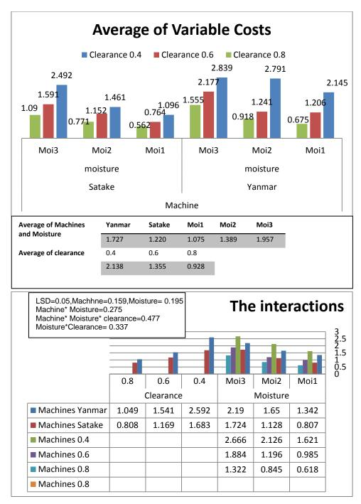
Fig (5) IIIustartes effect of machines types, Clearance and Grain moisture in the Average of Variable Costs \$\Ton.
