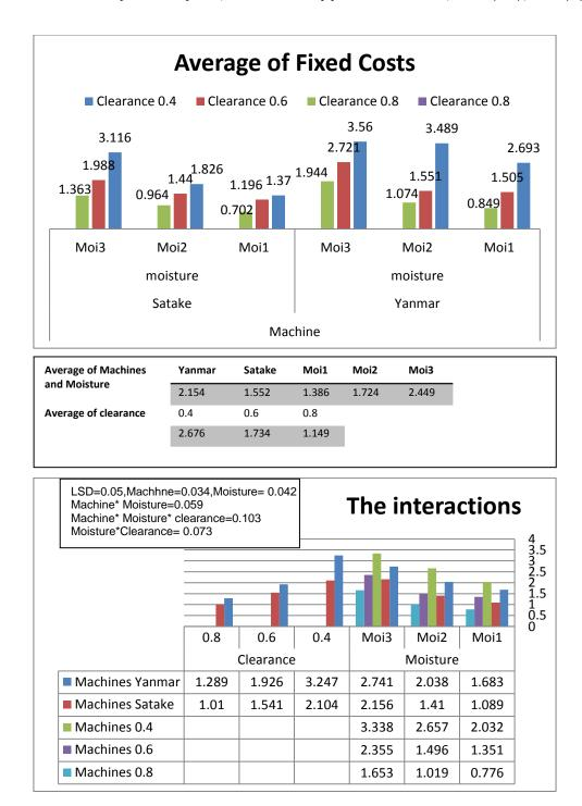
Fig (4) IIIustartes Effect of Machines types , Clearance and Grain Moisture in the Average of Fixed Costs \$\Ton.
