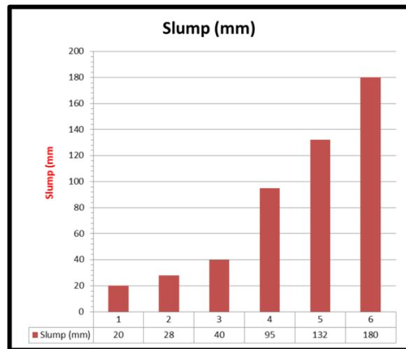
Figure. 3: slump with different (SP) mixing ratios
