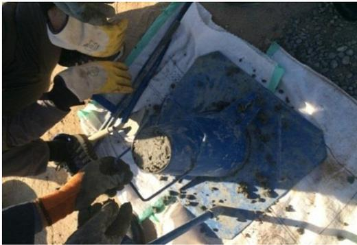
Figure. 1: slump test
