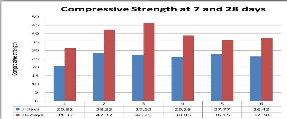
Figure.5 : compressive strength at 7 and 28 days for different (SP) mixing ratios
