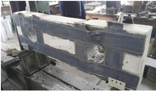
Plate 5: Failure mode and tearing of CFRP strip for B3-R-VH
