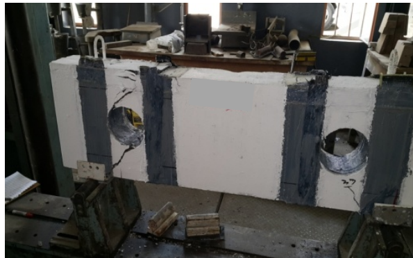
Plate 3: Failure mode and cracks patterns for B1-R-V
