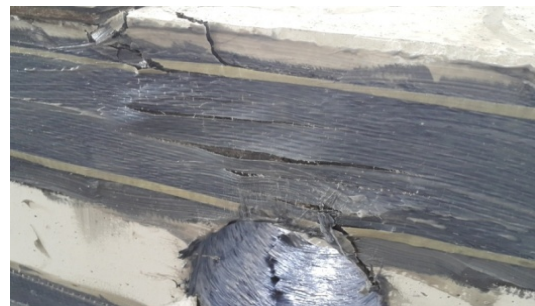
Plate 4: Failure mode and tearing of CFRP strip for B2-R-H
