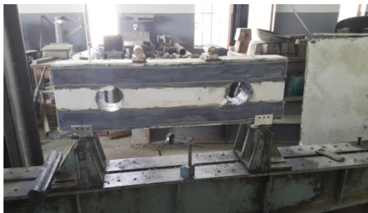
Plate 4: Failure mode and tearing of CFRP strip for B2-R-H
