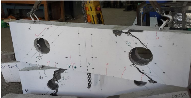
Plate 2: Failure mode and cracks patterns for B1-Control
