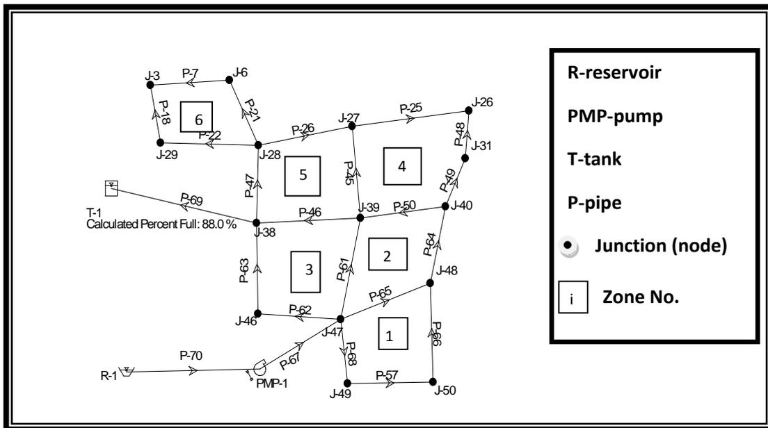
**Fig. (1) Direction of discharge in the pipes when the pump status is power on**
