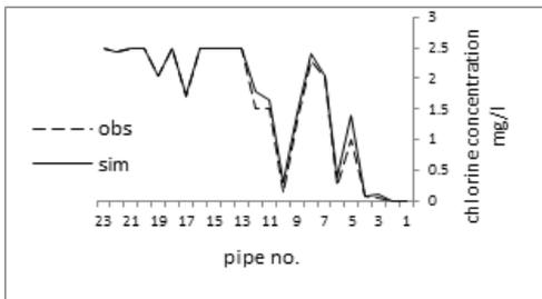
Fig.(9) Comparison between obs. and sim. chlorine conc. before calibration is done
