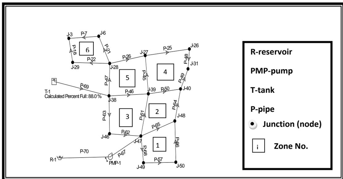
**Fig. (2) Direction of discharge in the pipes when the pump status is power off**
