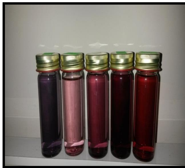
Figure 1: Colors variation during the synthesis process of gold nanoparticles (Trisodium citrate as reducing agent) Interaction equation.
