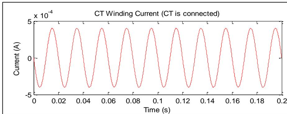
**Figure (8) CT Winding Current, CT 2000:5, 100VA, 4Ω, injected 20A**
