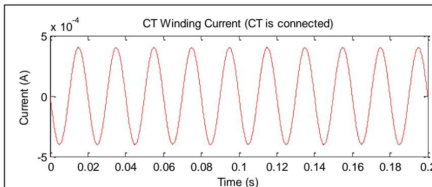
Figure (6) CT Winding Current, CT 1200:5, 100VA, 4Ω, injected 5A
