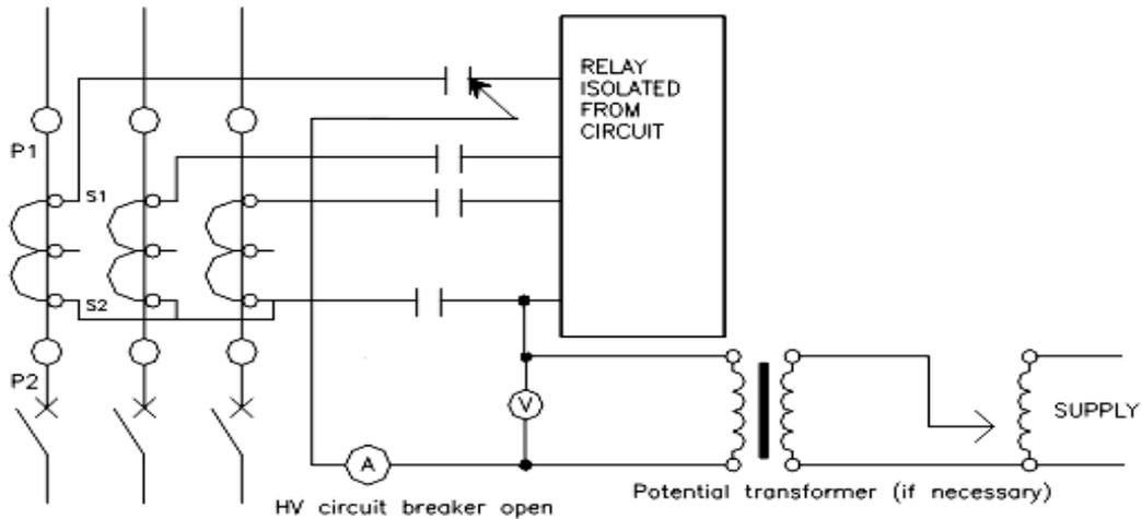
Figure (3) Secondary Injection Tests
