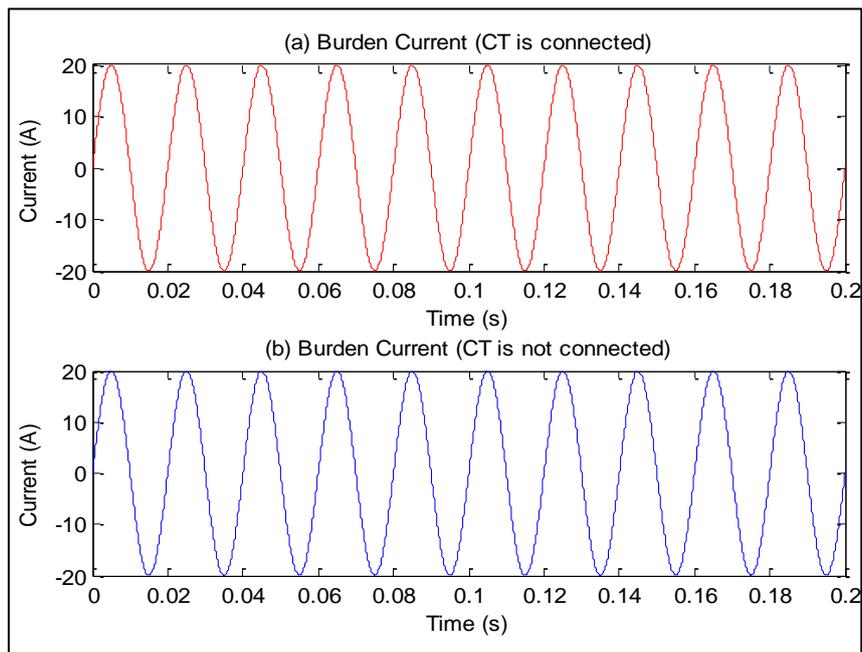
**Figure (11) Burden Current, CT 2000:5, 100VA, 4Ω, injected 20A**
