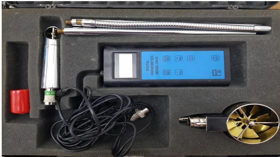
**Figure (7) digital air anemometer.**
