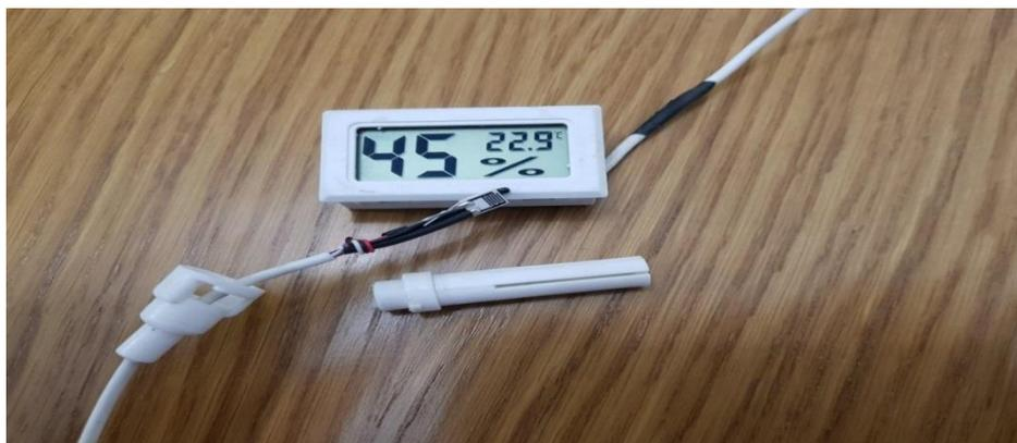
Figure (5) Digital Air Hygrometer & Thermometer
