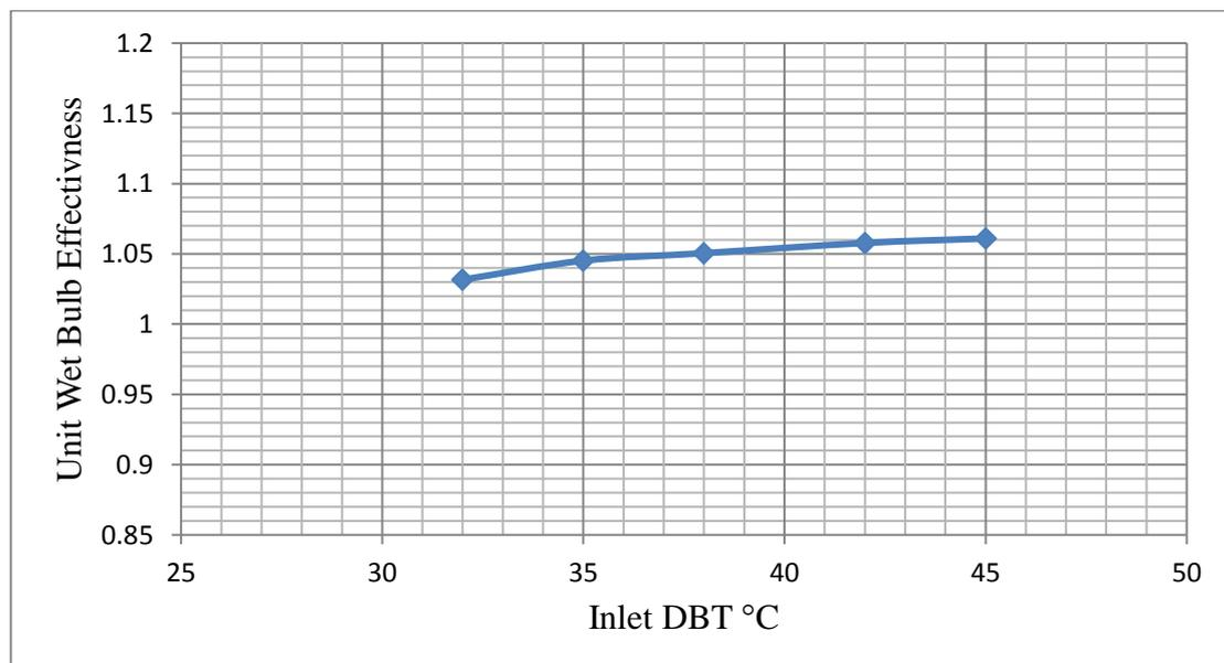
**Figure (14) Wet bulb effectiveness versus inlet air temperature (Inlet air volume flow rate = 0.425 m<sup>3</sup>/s, Inlet air humidity ratio = 5 g water/kg dry air, E.R. = 35%, water flow rate = 0.1 L/s)**
