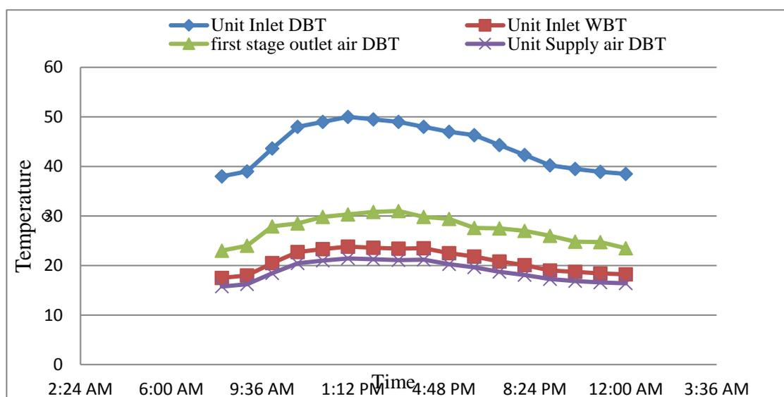
**Figure (12) Daily unit temperature readings with volumetric inlet air flow rate = 0.425 m<sup>3</sup>/s, H.E. Water flow rate = 0.1 L/s, E.R. = 0.35 %.**
