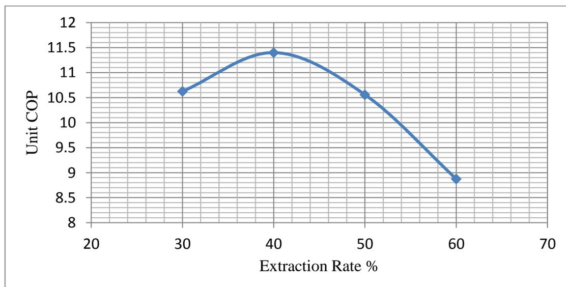
**Figure (16) Unit COP versus extraction rate % ( Inlet air DBT=38°C, Inlet air volume flow rate = 0.425 m<sup>3</sup>/s, Inlet air humidity ratio = 5)**
