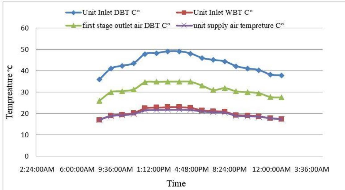
**Figure (13) Daily temperature readings when volumetric inlet air flow rate = 0.48 m<sup>3</sup>/s, H.E. Water flow rate = 0.1 L/s, ER = 0.35 %.**
