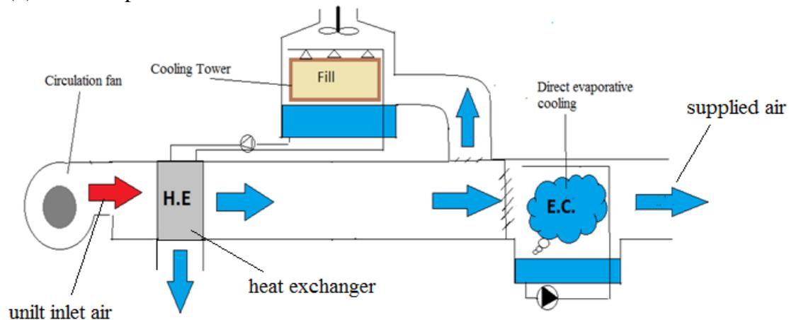
Figure (1) Combined system layout
