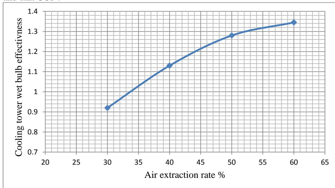
**Figure (15) Wet bulb effectiveness versus extraction rate % ( Inlet air DBT=38°C, Inlet air volume flow rate = 0.425 m<sup>3</sup>/s, Inlet air humidity ratio = 5g water/kg dry air).**
