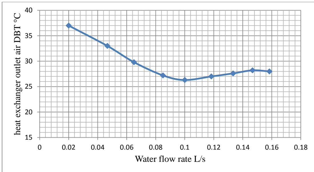
**Figure (11) the effect of water flow between the cooling tower and heat exchanger on heat exchanger outlet air DBT (Unit Inlet DBT= 40°C, inlet WBT = 20°C, inlet volumetric air flow rate = 0.425 m<sup>3</sup>/s, extraction rate = 35%).**
