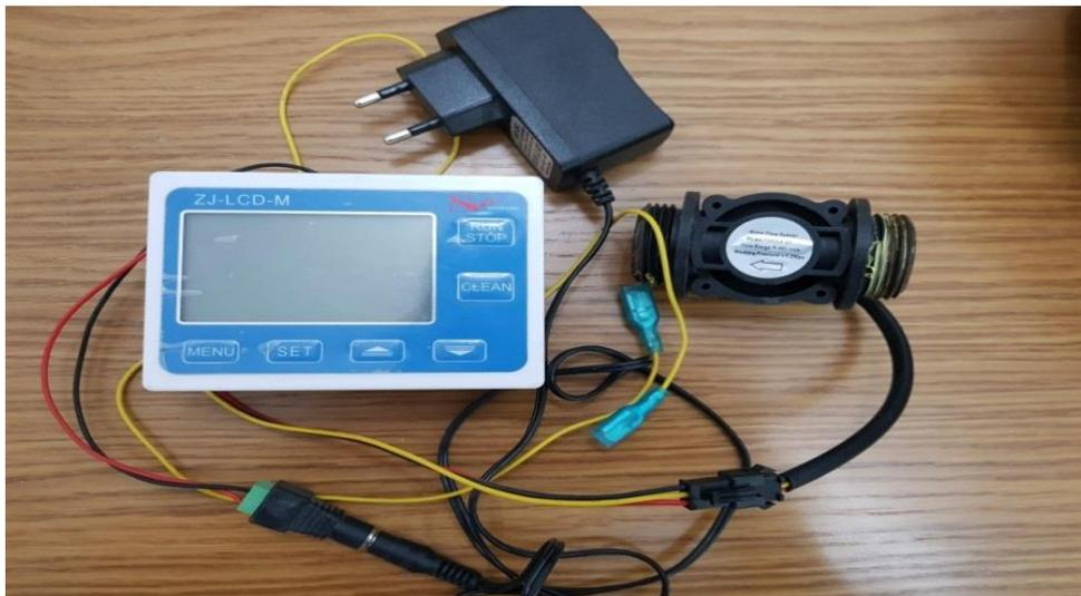
**Figure (8) the used water flow meter.**
