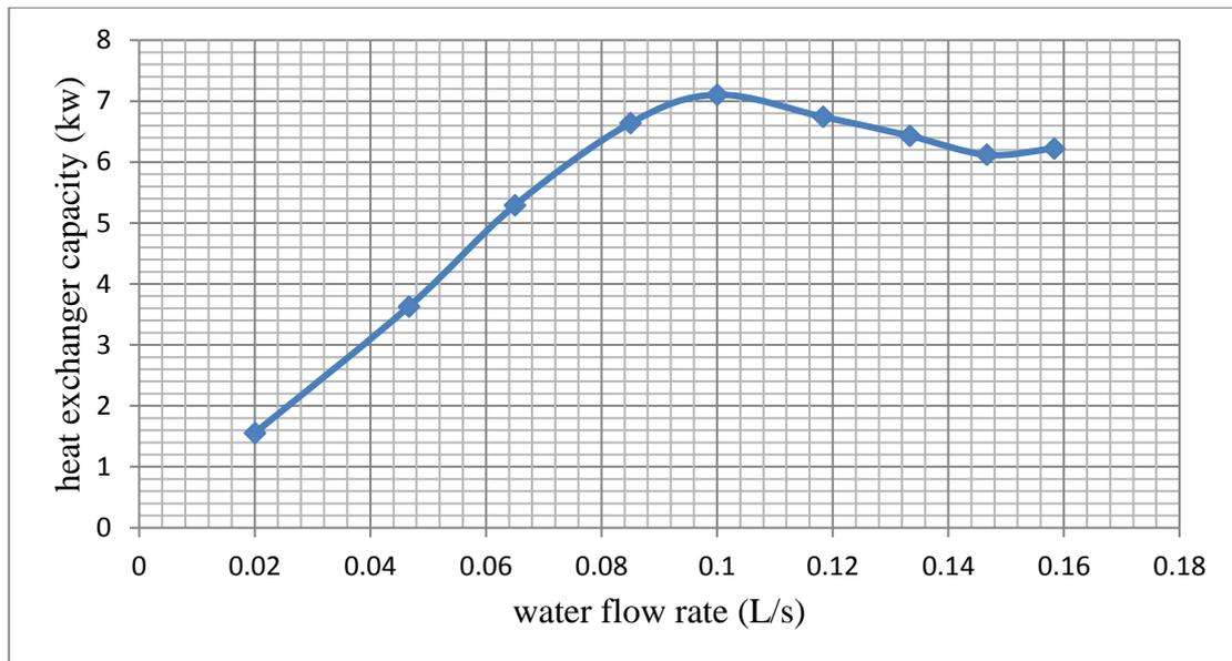
**Figure (9) the heat removed from the heat exchanger with various water flow rates , (Unit Inlet DBT= 40°C , inlet WBT = 20°C , inlet volumetric air flow rate = 0.425 m<sup>3</sup>/s ,extraction rate = 35%).**
