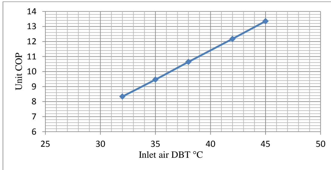
**Figure (17) Unit COP versus inlet air temperature (Inlet air volume flow rate =  $0.425 \text{ m}^3/\text{s}$ , Inlet air humidity ratio =  $5 \text{ g water/kg dry air}$  and extraction ratio =  $35\%$ )**
