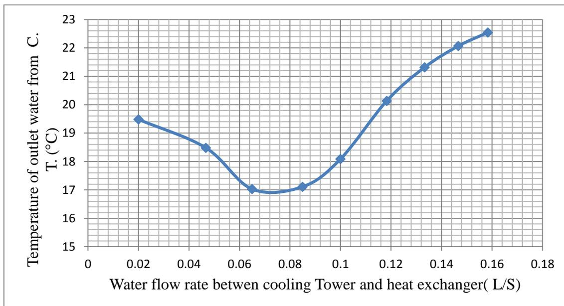
**Figure (10) the effect of water flow on cooling tower Water outlet temperature (Unit Inlet DBT= 40°C , inlet WBT = 20°C , inlet volumetric air flow rate = 0.425 m<sup>3</sup>/s, air extraction rate =35%).**
