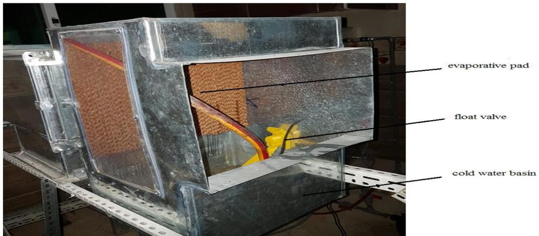
Figure (4) direct evaporative section
