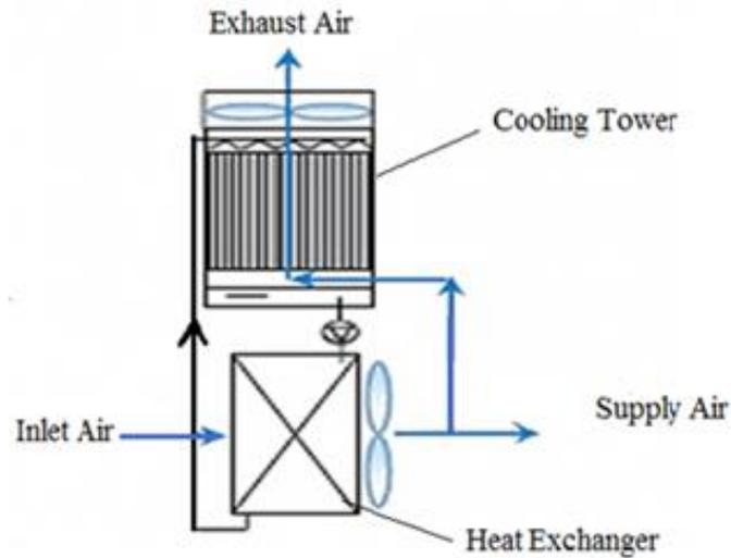
Figure (3) external regenerative indirect evaporative cooling
