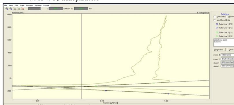
Figure 5: The polarization curve of the brass sample coated with epoxy and 3% wt of  $WO_3$  nanoparticles
