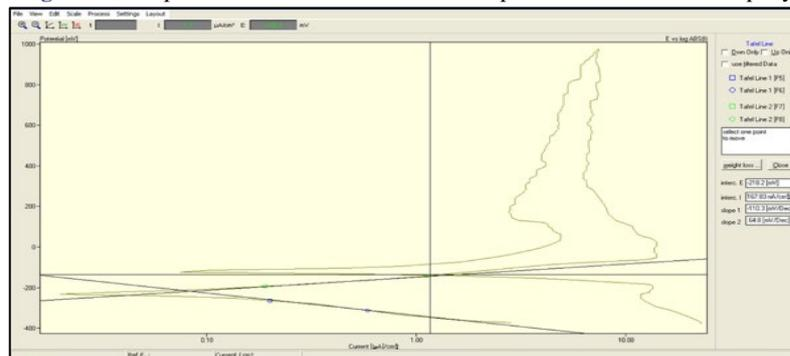
Figure 3: The polarization curve of the brass sample coated with epoxy and 1% wt of  $WO_3$  nanoparticles
