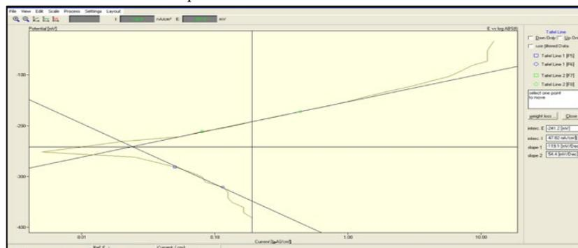
Figure 4: The polarization curve of the brass sample coated with epoxy and 2% wt of  $WO_3$  nanoparticles
