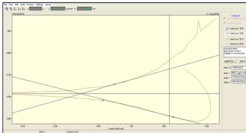
**Figure 1:** The polarization curve of the uncoated
