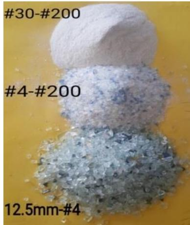
**Figure 1 Size of crushed waste glass**
