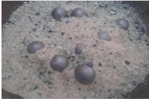
**Figure 3 Los Angeles abrasion for glass sample.**
